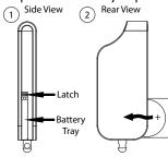
Using a small flat narrow object, push latch down towards battery tray while gently prying the tray outwards from both ends until released. Remove the tray from the remote control housping.
