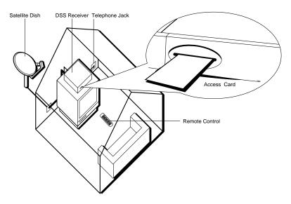
DSS<sup>®</sup> Satellite Dish Antenna Picks up the satellite's coded program information and relays it to your DSS<sup>®</sup> receiver. (Your satellite dish may be installed in different locations on or around your house. The satellite dish antenna must, however, be pointed in a southern direction toward the satellite.)
