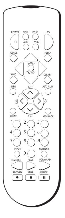
**INPUT** In TV and VCR mode, press the INPUT button one or more times to toggle through the available video inputs.
