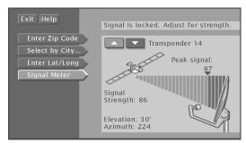
If the dish is pointed to the correct azimuth and elevation, the signal meter will show you the current signal strength (and you should hear a continuous tone).
