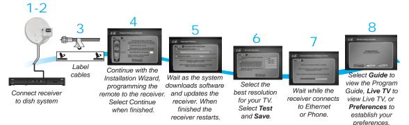
1 Connect one RG-6 coaxial cable from the LNBF to a DISH Pro Plus (DPP) Separator or a DISH Pro Plus Triplexer. Connect the DPP Separator or DPP Triplexer to the SATELLITE IN port on the receiver's back panel.
