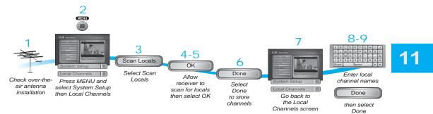
1 Verify your over-the-air antenna is installed and connected to the receiver's **OVER-THE-AIR ANTENNA IN.**
