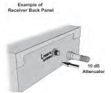
3 Attach the remote control antenna to the attenuator.
