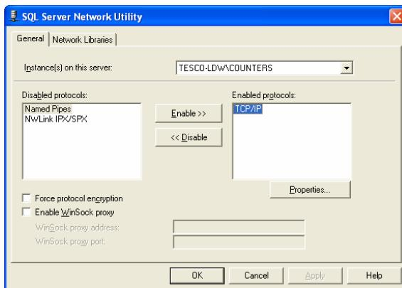
Select the correct instance and enable TCP, as above. This need to be configured on both Instances. Once configured reboot machine.
