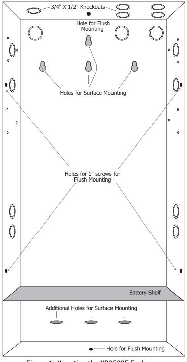
Figure 1: Mounting the XR2500F Enclosure
