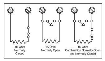
Figure 12: Protection Zone Wiring
