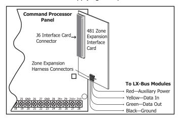
Figure 6: 481 Wiring
