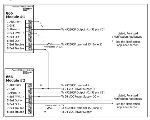
Figure 5: 866 Modules Wiring
