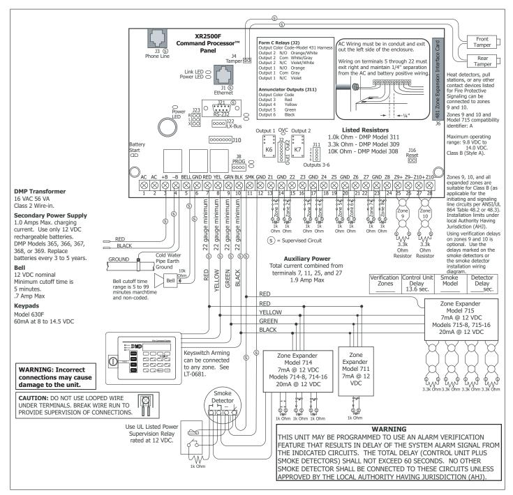
Figure 12: Typical XR2500F Wiring Diagram
