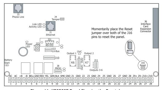
Figure 16: XR2500F Panel Showing the Reset Jumper
