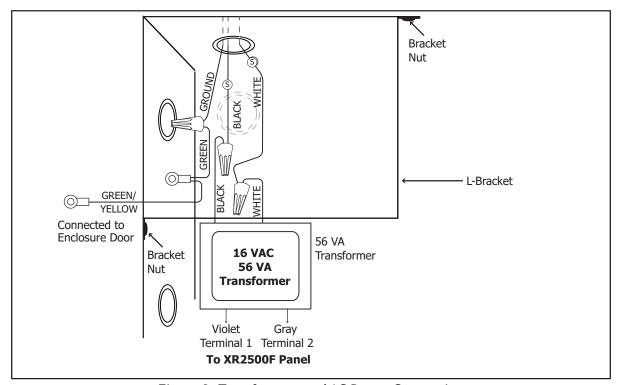
Figure 3: Transformers and AC Power Connection
