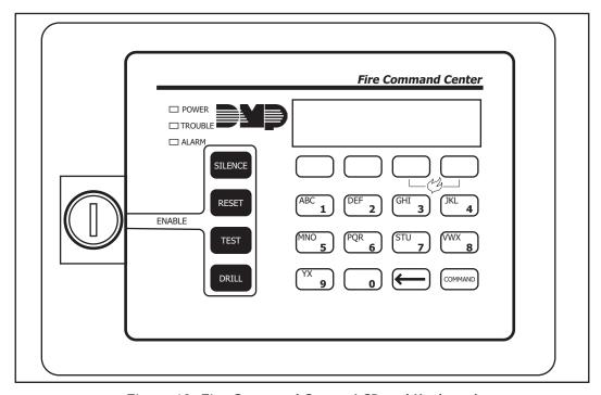
Figure 10: Fire Command Center LCD and Keyboard
