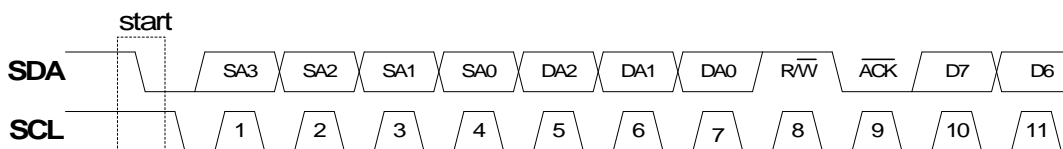
Figure 13-5. Addressing an I2C Peripheral
