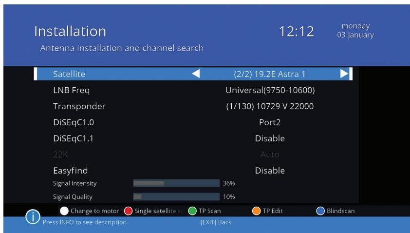
Press the white button to select how to set the antenna to the LNB.
