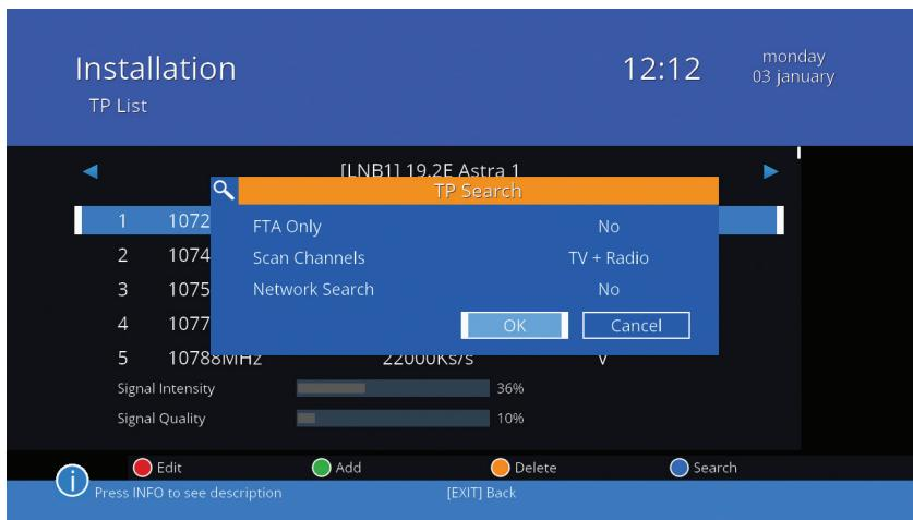
**● TP search** **Transponder scan.** Press the green button to scan the transponder. In the window that appears after 3 seconds on the screen, set the options:
