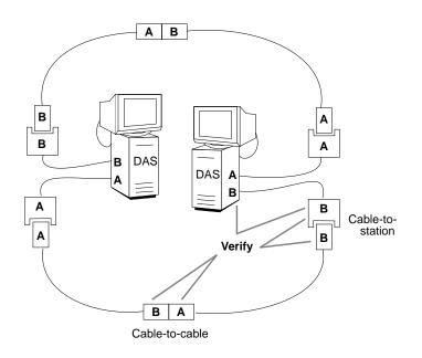
Figure 4-2 Correct Cable Connections
