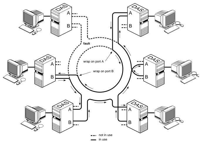
Figure 3-5 Fault Isolation and Ring Wrap
