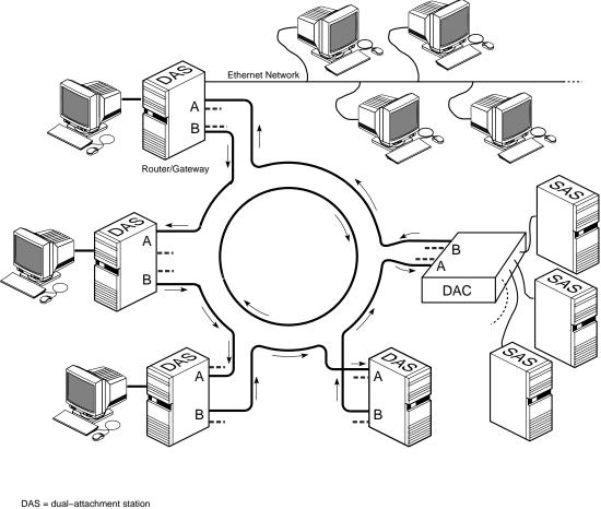
DAS = dual-attachment station SAS = single-attachment station DAC = dual-attachment concentrator
