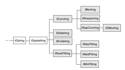
Figure 4-13 Spatial Domain Operator Inheritance Hierarchy
