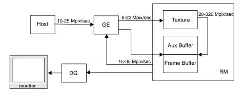
**Figure 7-2** RealityEngine Pixel Transfer Paths (transfer rates are in millions of pixels per second)
