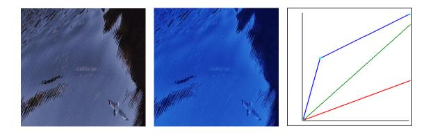
Figure D-26 ilLutImg (original, filtered image, and LUT editor)
