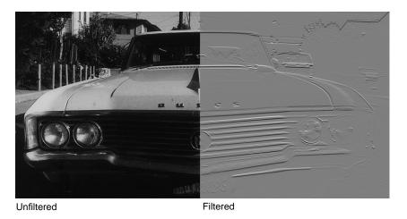
Figure 4-22 A Compass Filtered Image
