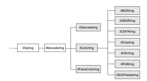
Figure 4-2 Color Conversion Operators Inheritance Hierarchy
