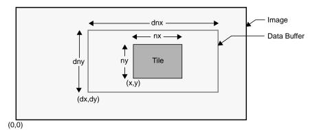
Figure 2-9 Parameters for getSubTile() and setSubTile()
