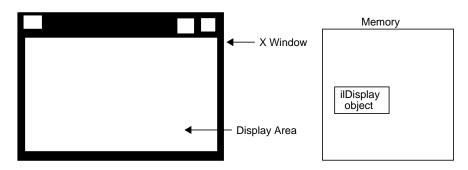
Figure 5-3 ilDisplay Object Creates a Display Area
