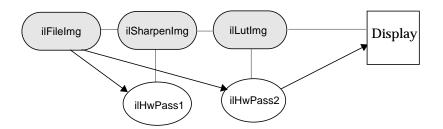
Figure 7-4 Composite Operation
