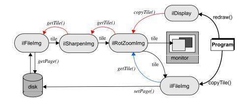
Figure 2-11 Image Chain Showing Demand-driven Execution Model
