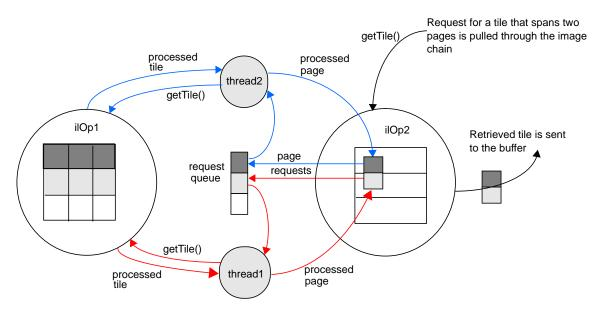
Figure 2-13 Operators, Requests for Pages, and Threads
