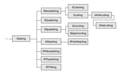
Figure 6-2 ilOpImg and Its Subclasses for Deriving
