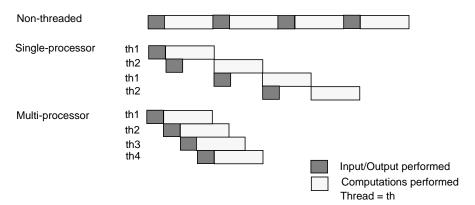
**Figure 2-13** Performance Comparison of Non-threaded, Single-processor, and Multi-processor Applications
