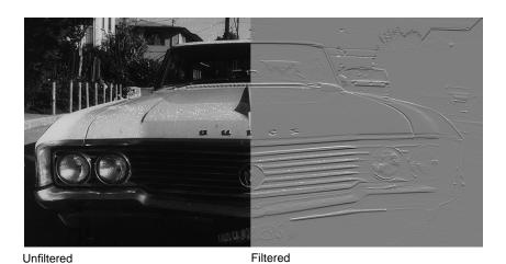
Figure 4-22 A Compass Filtered Image
