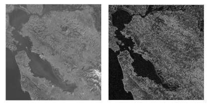
Figure H-21 ilSobelImg (original and filtered image)
