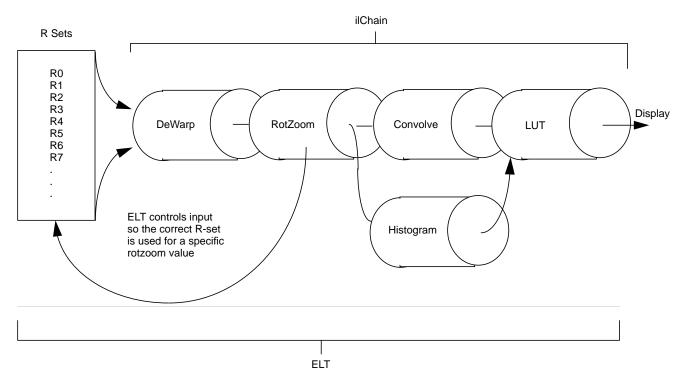
**Figure G-1** ELT image processing pipeline
