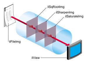
Figure 7-3 IL Chain Mapped to the OGLIP Pipeline
