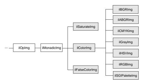
Figure 4-2 Color Conversion Operators Inheritance Hierarchy
