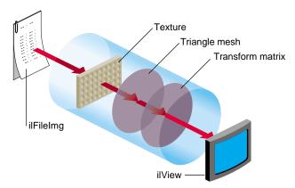
**Figure 7-8** Data Path of the IL Chain in Figure 7-7
