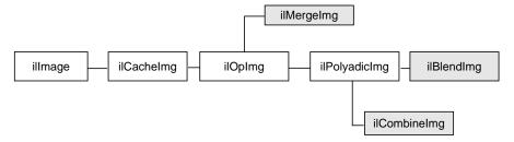
Figure 4-32 ilBlendImg, ilMergeImg, and ilCombineImg Inheritance Hierarchy
