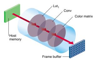
**Figure 7-4** Mapping onto the OGLIP in a Single Transfer
