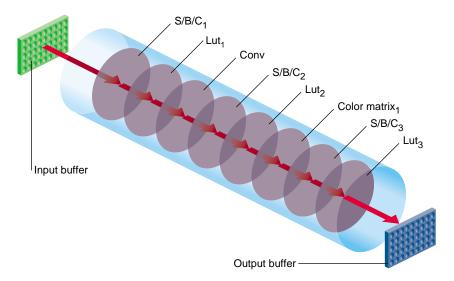
**Figure 7-2** OpenGL Image Processing Pipeline
