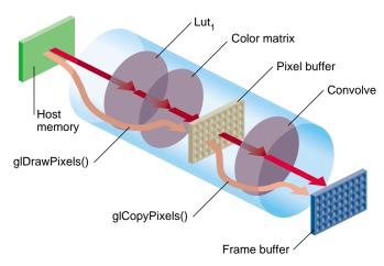
Figure 7-6 Two-Pass Transfer Operations
