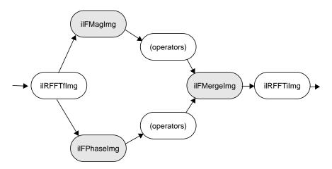
Figure 4-24 Magnitude and Phase Fourier Operators
