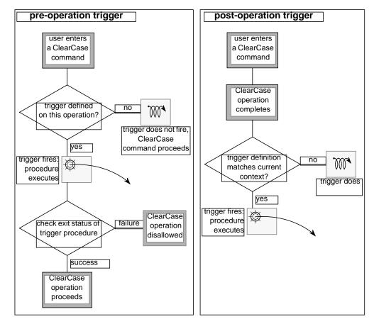
Figure 6-4 Pre-Operation and Post-Operation Triggers
