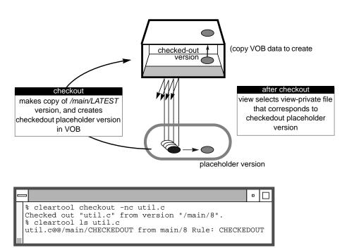
Figure 4-10 After a Checkout
