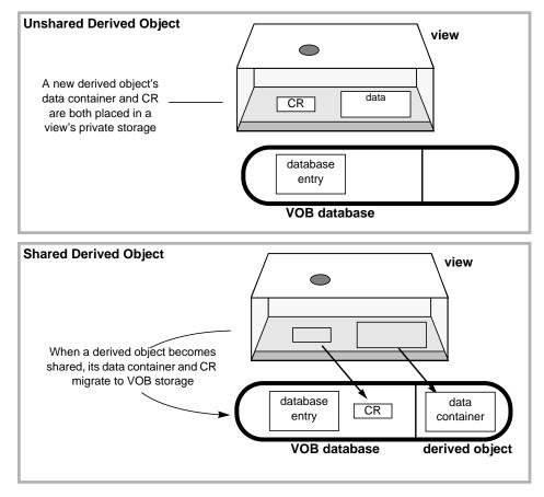
Figure 5-4 Storage of Derived Objects and Configuration Records
