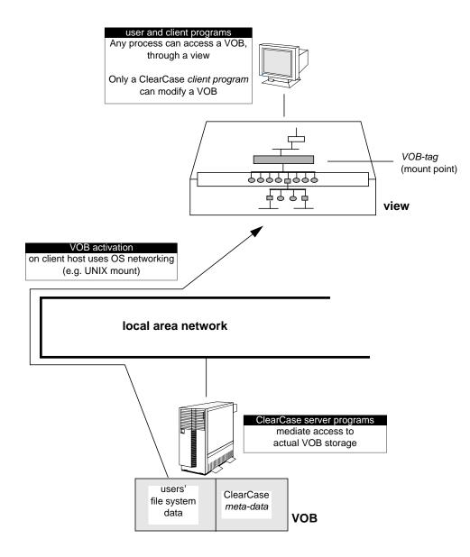
Figure 2-1 How ClearCase Users Access a VOB
