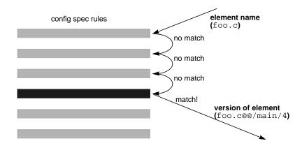
Figure 4-6 Using a Config Spec to Select a Version of an Element
