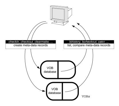
Figure 3-1 Meta-Data: ClearCase-Generated Records
