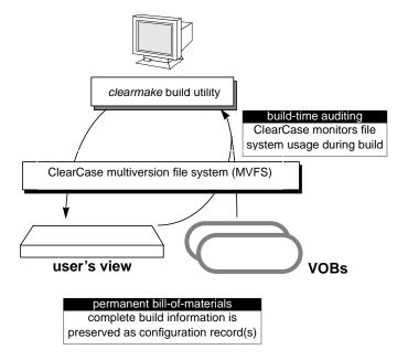
Figure 1-10 Build Auditing and Configuration Records
