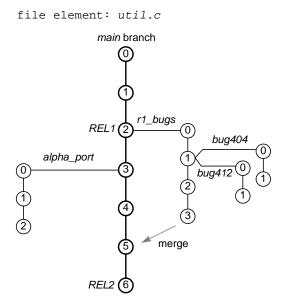
Figure 1-3 Version Tree of an Individual Element
