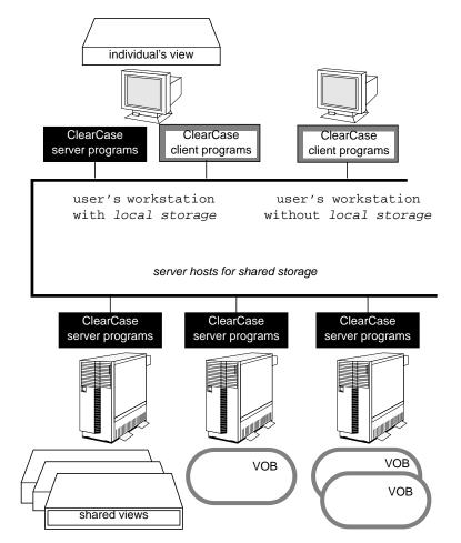
Figure 1-12 ClearCase Distributed Client-Server Architecture
