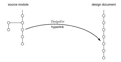
Figure 3-5 Hyperlink for Requirements Tracing
