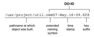
Figure 5-2 Extended Pathname of a Derived Object — DO-ID
