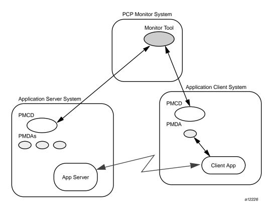
Figure 38. PCP Deployment to Measure Client-Server Quality of Service
