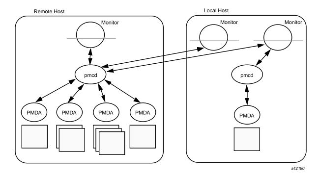
Figure 2. Process Structure for Distributed Operation
