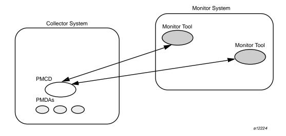
Figure 36. Basic PCP Deployment for Two Systems
