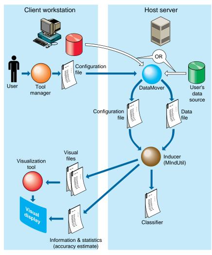
Figure 8-5 Tool Execution Sequence for Classifiers
