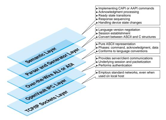
Figure 2-1 Communication Layers
