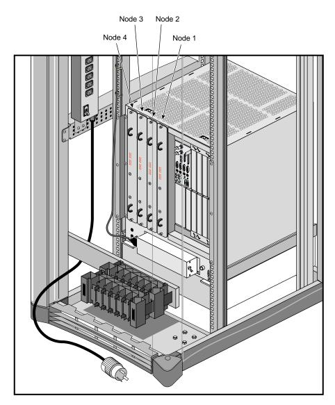
Figure 2-8 Node Board Positions in the Chassis
