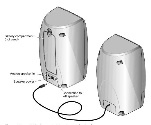
Figure 3-22 Cable Connection Locations on the Speakers
