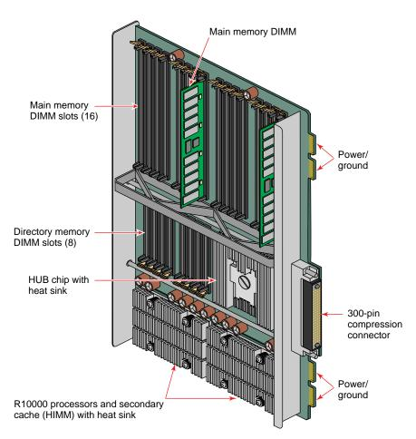
Figure 1-6 Node Board Example
