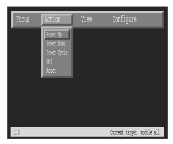
Figure 4-7 Multimodule System Controller Power Up Selection
