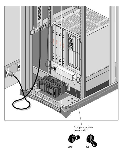
Figure 4-6 Powering On a Processor Compute Module
