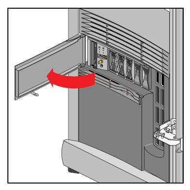
Figure 5-3 Opening the Compute Module's Door
