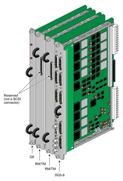
Figure 2-4 Graphics Pipes in the Module
