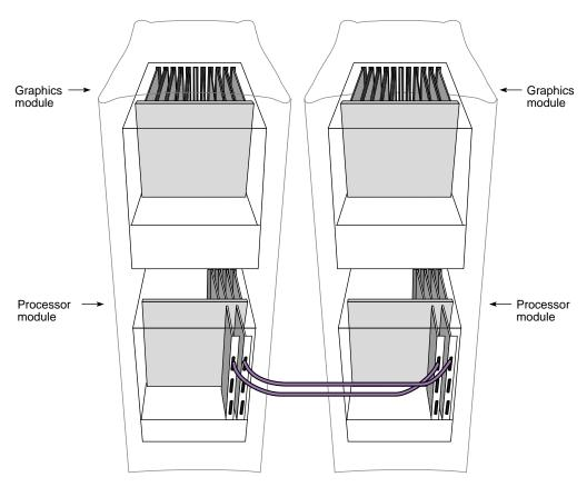
Figure 3-2 Onyx2 Multirack System (With 16P and 4 Graphics Pipes)
