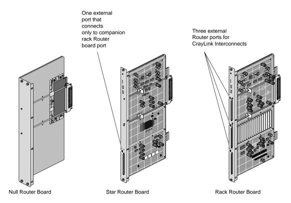
Figure 2-11 Types of Router Boards
