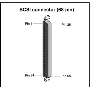
Figure 3-21 68-Pin Single-Ended SCSI Connector
