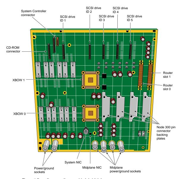
Figure 1-7 Processor Compute Module Midplane
