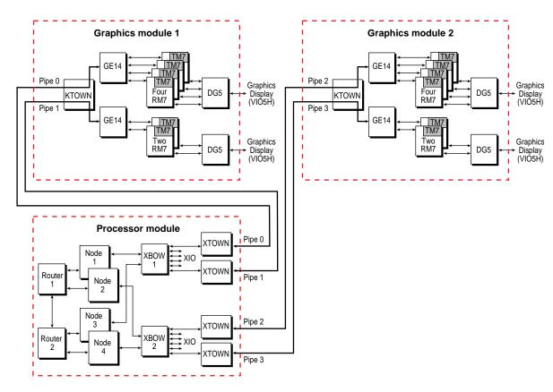
**Figure 1-5** Multirack Four-Pipe Diagram Example
