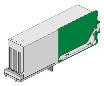
Figure 2-13 Optional PCI Board Carrier Assembly
