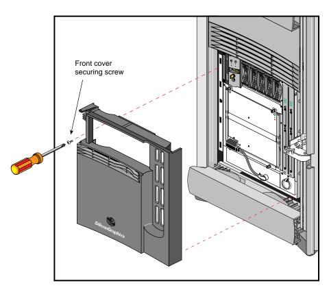
Figure 5-6 Removing the Compute Module's Facade
