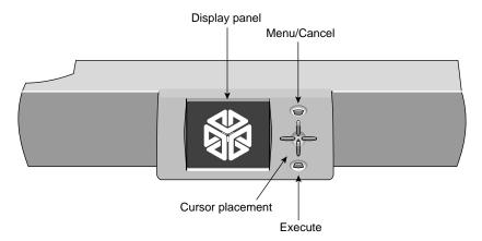
Figure 2-10 MMSC Interface and Display Panel
