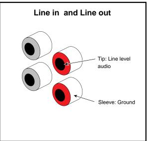
Figure 3-16 Line In and Out Stereo Ports
