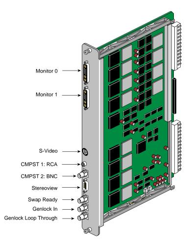
Figure 3-5 DG5-2 Graphics Panel Connections (Without Options)
