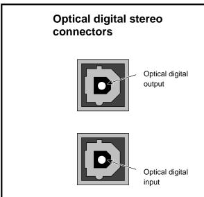
Figure 3-19 Optical Digital Audio Interface
