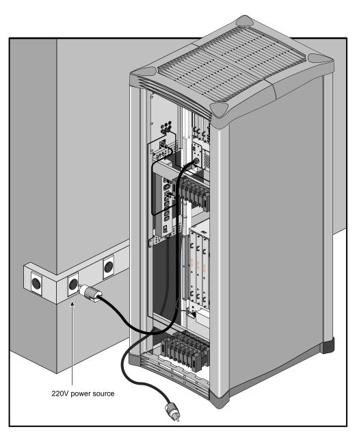
Figure 4-2 Connecting a Graphics Module Power Cable
