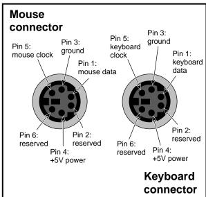
Figure 3-15 Keyboard and Mouse Locations and Pinouts
