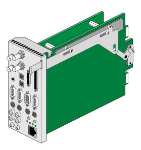
Figure 3-12 BaseIO (IO6G) Assembly and Connectors
