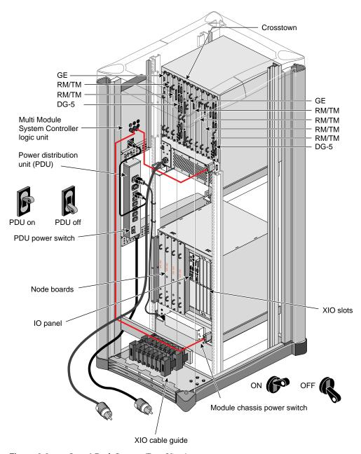
Figure 2-2 Onyx2 Rack System (Rear View)
