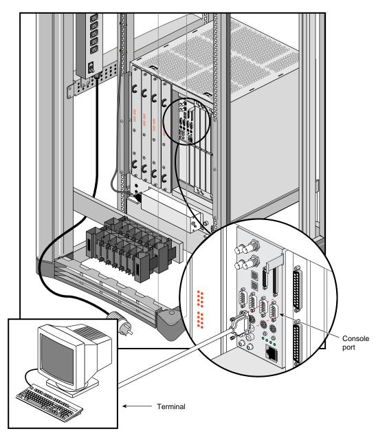
**Figure 3-18** Serial Port Connection Example
