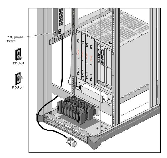
Figure 4-5 Turning On the PDU
