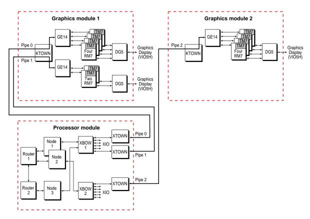
**Figure 1-4** Multirack Three-Pipe Diagram Example
