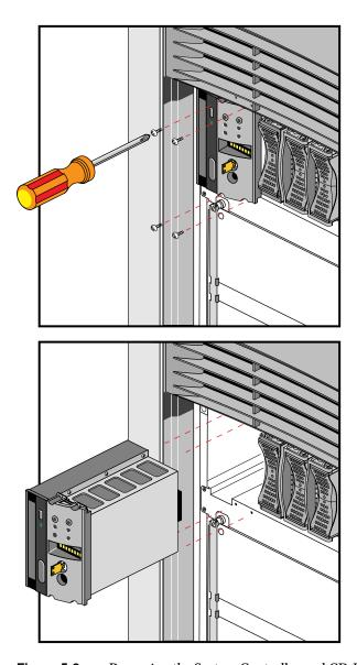
Figure 5-8 Removing the System Controller and CD-ROM
