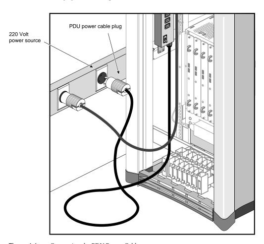
Figure 4-4 Connecting the PDU Power Cable
