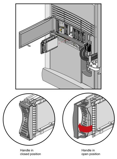
Figure 5-5 Removing the Drive
