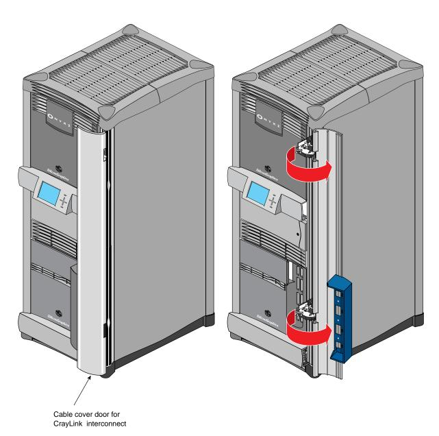
**Figure 5-2** Opening the Cable Cover Door
