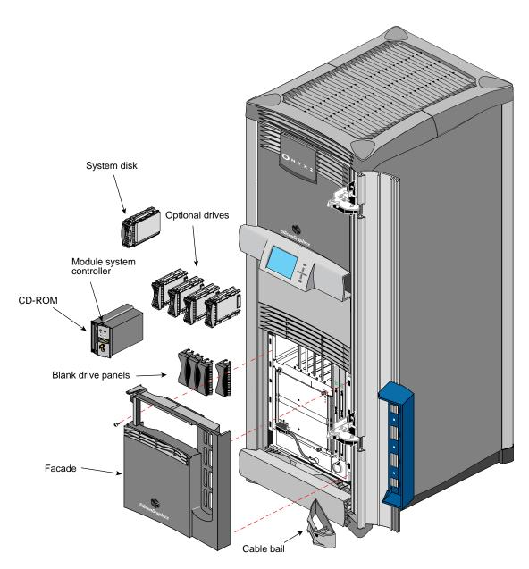
Figure 5-1 Onyx2 Rackmount Customer-Replaceable Units
