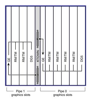
Figure 2-3 Graphics Module Pipes Diagram
