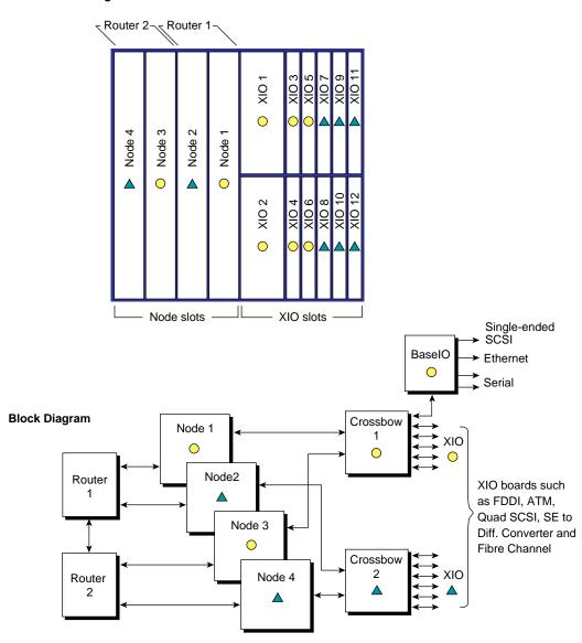
Figure 2-5 Block Diagram for the Compute Module (Single Rack)
