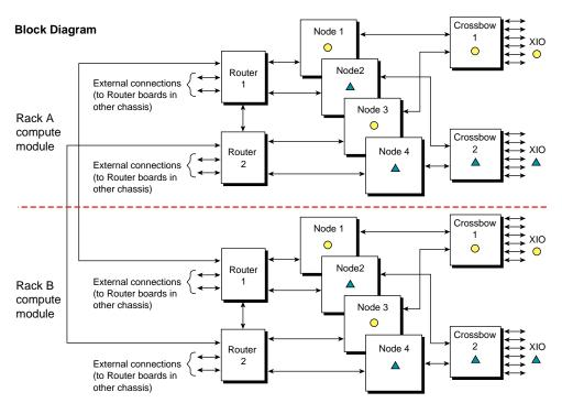
Figure 2-6 Block Diagram for the Compute Modules (Multirack System)
