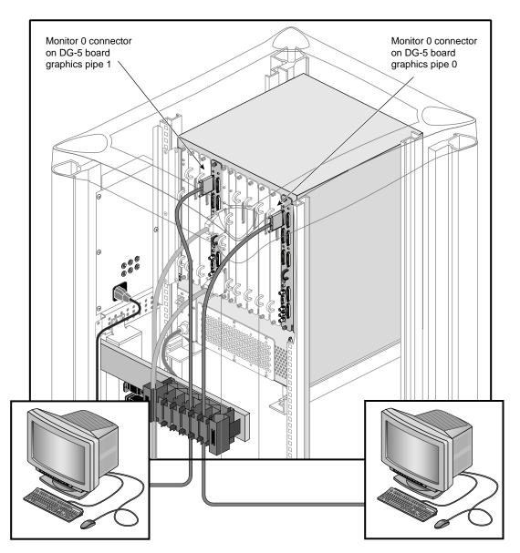
Figure 3-11 shows a connection example with two monitors attached to separate graphics pipes on the Onyx2 rack's graphics module.
