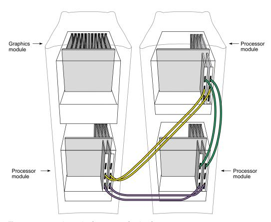
Figure 3-3 24P Onyx2 Configuration With 2 Graphics Pipes
