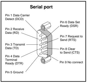
Figure 3-17 RS-232/RS-422 Serial Connectors
