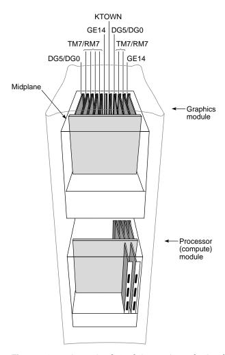
Figure 3-1 Onyx2 Single-Rack System (8P and 2 Graphics Pipes)
