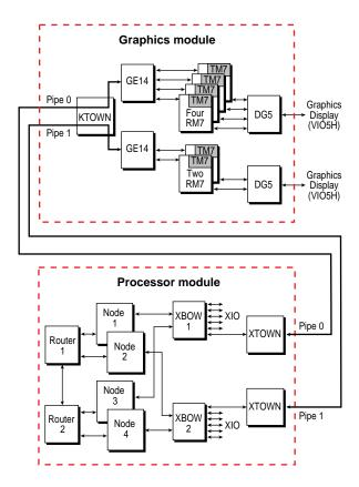
Figure 1-2 Single Rack Graphics Block Diagram Example
