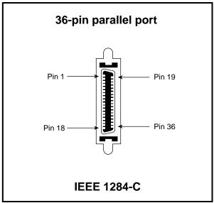
**Figure 3-14** Parallel Printer Port Location
