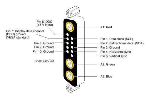
Figure 3-7 DG5/VIO5H 13W3 Connector Pinout
