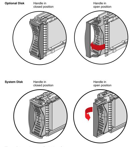
**Figure 5-4** Opening the SCA Disk Drive Units
