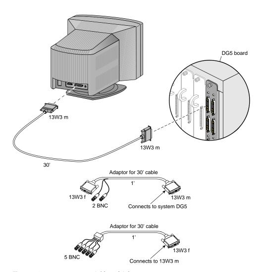
Figure 3-10 13W3 Monitor Cable and Adapters
