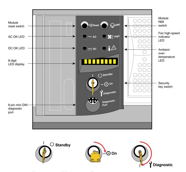
Figure 4-3 Module System Controller Key Positions
