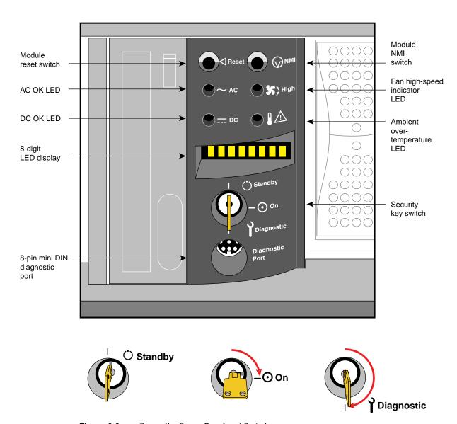
Figure 6-3 Controller Status Panel and Switches
