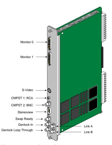
Figure 3-8 DG5 With Optional GVO Connectors
