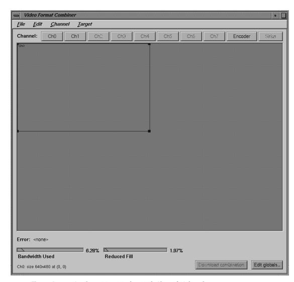
Figure A-2 shows the main window with Channels 0 and 1 in the managed area.
