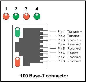
**Figure 3-13** 10/100 Base-T Ethernet Connector
