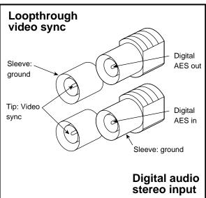
Figure 3-20 Loopthrough and Digital Audio Connectors
