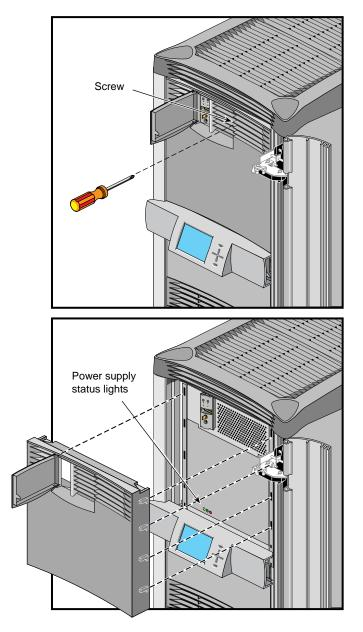
Figure 5-7 Removing a graphics Module Facade
