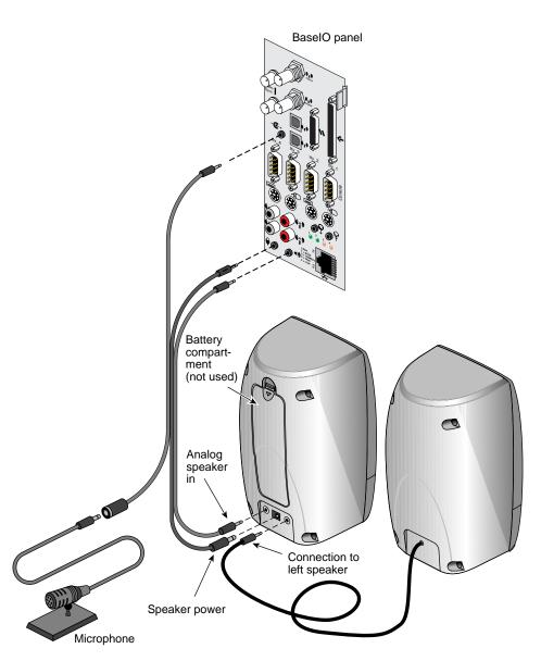
Figure 3-23 Speaker and Microphone Connections to the BaseIO
