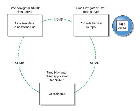
Figure F-1 NDMP Three-way Architecture
