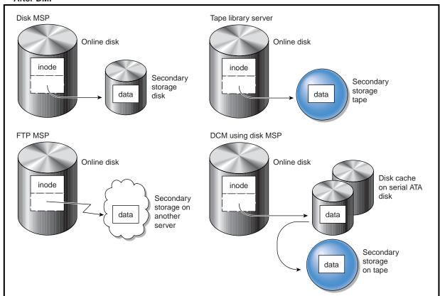
Figure 1-2 DMF Mechanisms
