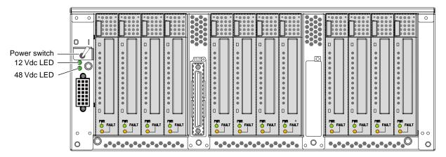
**Figure 2-7** Power Switch at the Rear of the Module
