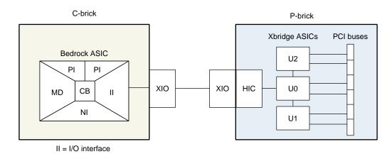
Figure 3-2 P-Brick Block Diagram
