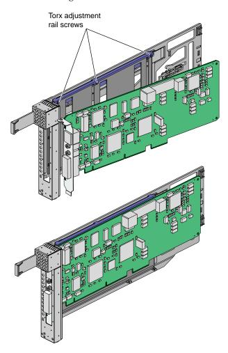
Figure 2-4 Mounting PCI Card Into Carrier
