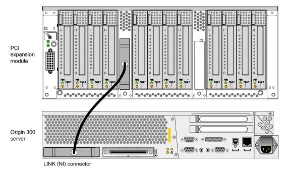
**Figure 1-8** Cabling a PCI Expansion Module to an Origin 300 Server
