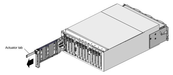
Figure 2-1 Removing a PCI Card Carrier
