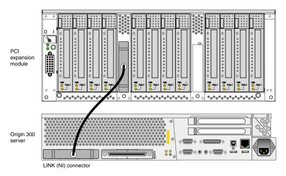
Figure 3-14 Origin 300 Server to PCI Expansion Module Configuration
