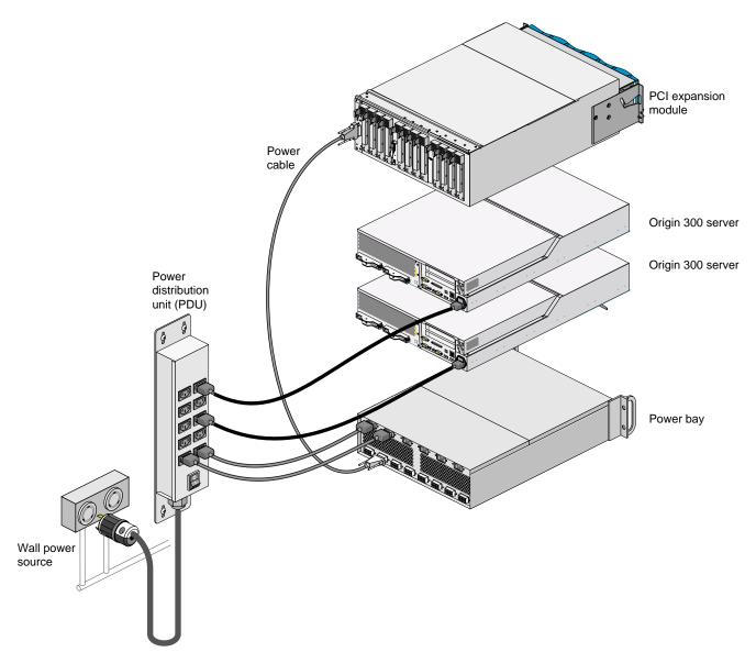
Figure 1-11 Cabling the PCI Expansion Module to the Power Bay
