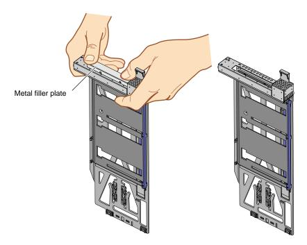
**Figure 2-3** Extracting PCI Carrier's Metal Filler
