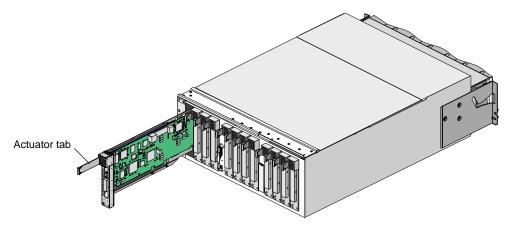
Figure 2-5 Installing a PCI Card in a PCI Slot
