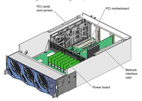
Figure 3-8 Internal View of PCI Expansion Module
