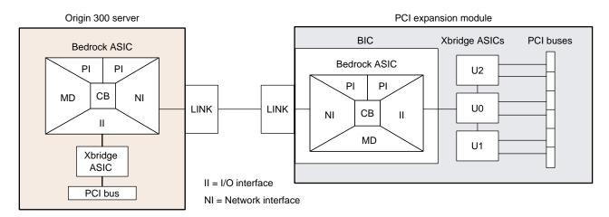
Figure 3-3 PCI Expansion Module Block Diagram
