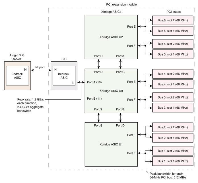
Figure 3-5 PCI Expansion Module Block Diagram
