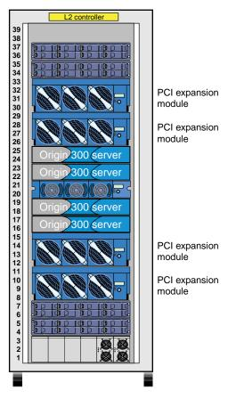
Figure 1-3 Placement of PCI Expansion Module (Tall Rack with NUMAlink Module)
