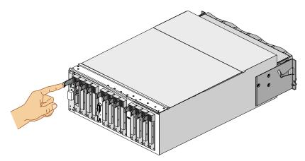
**Figure 2-6** Seating the PCI Card in the PCI Slot
