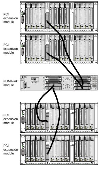
Figure 3-14 shows four PCI expansion modules connected to a NUMAlink module.
