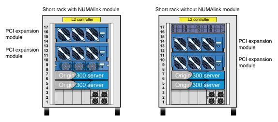
**Figure 1-2** Placement of PCI Expansion Module (Short Rack)
