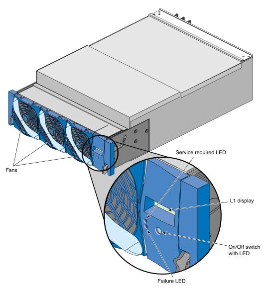
Figure 3-6 Front View of PCI Expansion Module
