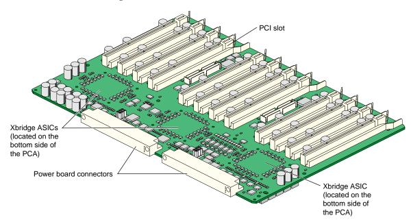
Figure 3-9 PCI Motherboard
