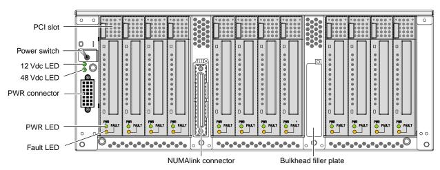
Figure 3-7 Rear View of PCI Expansion Module
