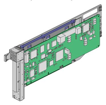
Figure 3-10 PCI Carrier with PCI Card Installed
