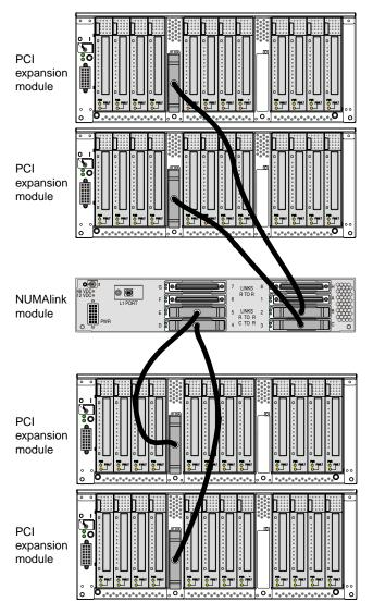
Figure 1-9 Cabling PCI Expansion Module to NUMAlink Module (Tall Rack)
