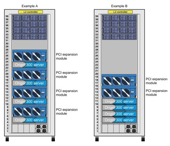
Figure 1-4 Placement of PCI Expansion Module (Tall Rack without NUMAlink Module)
