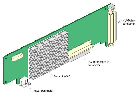
Figure 3-12 Bedrock Interface Card
