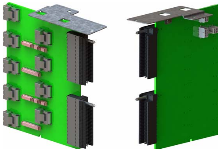
Figure 1-31 MIS JBOD Midplane I/O Connector (right & left views)
