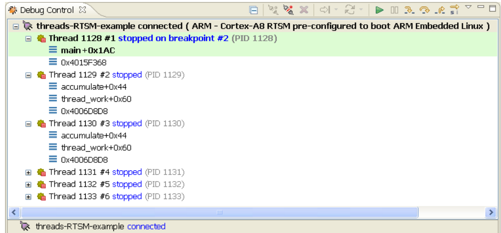
Figure 24-1 Threading call stacks in the DS-5 Debug Control view
