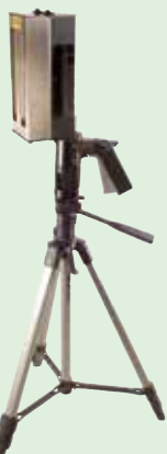
No. KSSPG used to tripod-mount a Shortwave UV Light source.
