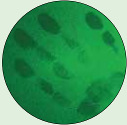
Untreated latent print on a metal filing cabinet as it may appear through the CYCLOPS Imager.
