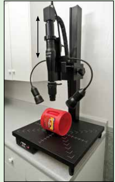
Larger objects of interest can be scanned for prints by both raising the RUVIS imager and extending it's distance from the Labkam's copy stand column.
