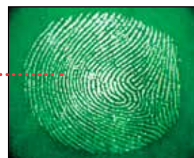
Cyanoacrylate-fumed fingerprint on the same soft drink can be photographed with a digital camera connected to the KRIMESITE™ IMAGER. No background colors!
