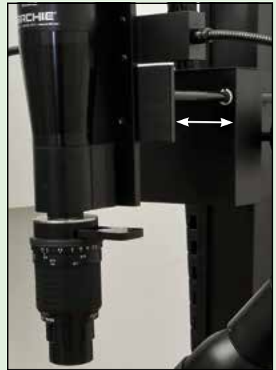
Close-up showing movement of RUVIS imager toward and away from LABKAM copy stand column.
