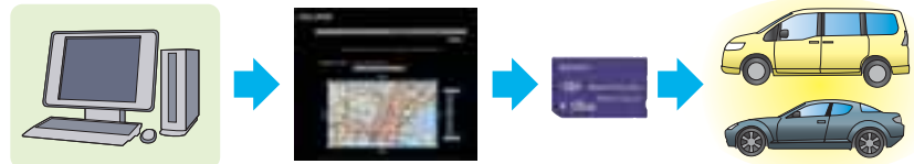
Routes can be set by accessing ECLIPSE's E-ISERV server. Map data is then downloaded onto a Memory Stick Duo which can be input into the AVX5000.
