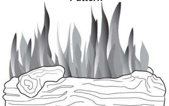
Figure 17 - Incorrect Burner Flame Pattern When Using Wrong Gas Type
