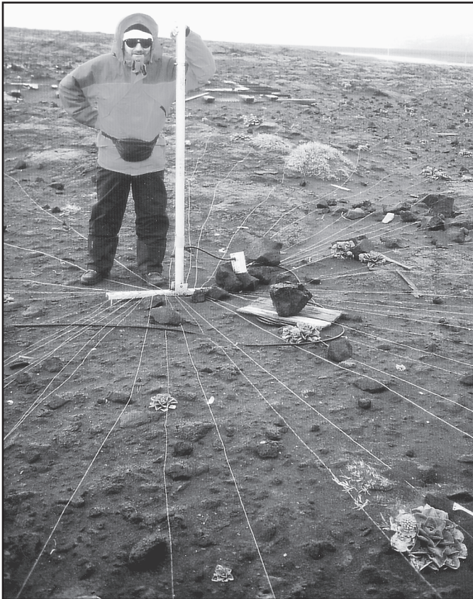
Fig 9-21—The Battle Creek Special that made Heard Island available on 160 for over 1000 different stations. Ghis, ON5NT, is not holding up the antenna; it is very well capable of standing up by itself. The antenna was located near the ocean's edge, on saltwater-soaked lava ash.
