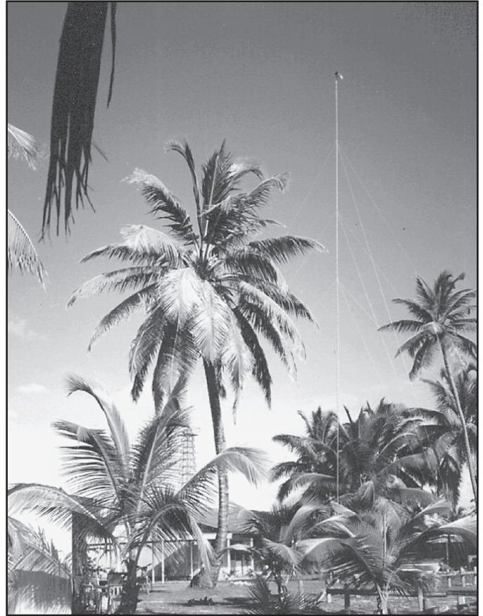
Fig 9-102—The Titanex V160E antenna on the beach on VK9CR, surrounded by beautiful coconut trees. This 26.8-meter-long special DXpedition vertical weighs only 7.5 kg and disassembles into 2.1-meter long sections, ideal for traveling!
