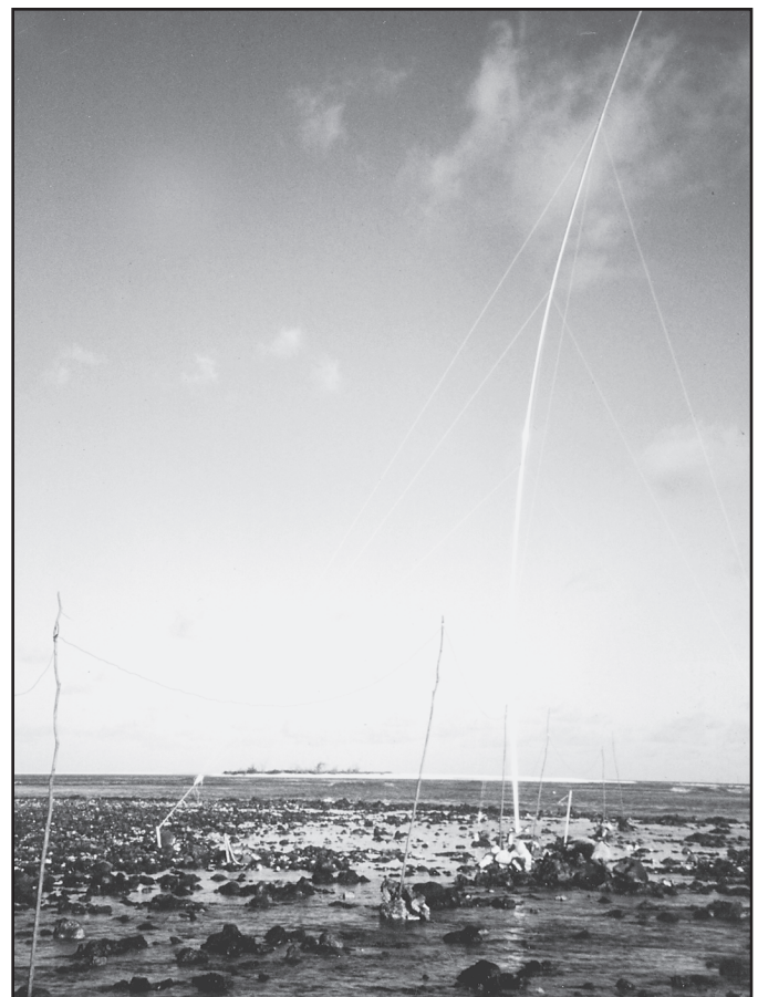
Fig 9-40—The Titanex V160E antenna on the beach at 3B7RF (St Brandon Island). Note the two elevated radials about 2 meters above salt water. The combination of one or two elevated radials with a perfect ground underneath is hard to beat.
