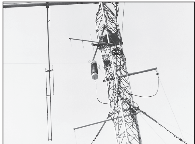
Fig 9-93—The K9RJ coaxial trap feeds a 160-meter inverted V hanging from the top of a tower, which is also used as a shunt-fed vertical for 160 meters. The entire construction looks somewhat like an oversized center insulator or balun.
