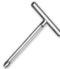
**Turf Coring Tool** — Turf style installation tool for shallow sensor installation depths, to 12" (30 cm). Nickel plated 7/8" (22 mm) soil coring tool with integral handle. Can also be used for soil sampling.
