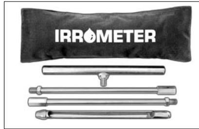
**Coring Tool Kit** — Nickel plated 7/8" (22 mm) soil coring tool. Comes as a kit in fabric storage pouch with two 12" (30 cm) extensions and handle for making up to a 36" (90 cm) access hole. Can also be used for soil sampling.
