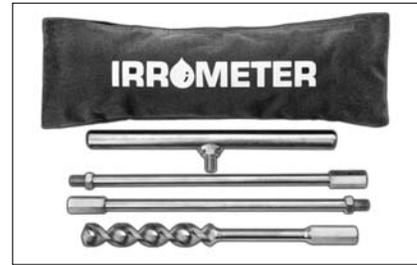
**Auger Tool Kit** — Nickel plated 1" (25 mm) soil auger. Makes oversize hole for grout style sensor installation in hard or rocky soils. Comes as a kit in fabric storage pouch with two 12" (30 cm) extensions and handle for making up to a 36" (90 cm) access hole.
