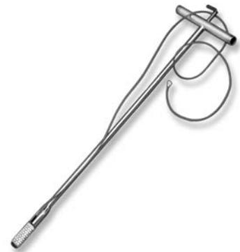
**WATERMARK Insertion Tool** — WATERMARK Sensor insertion tool. Tee handle style tool for inserting the WATERMARK Sensor up to 30" (76 cm) into the borehole created by one of the tools shown here. Has internal ejection rod inside tube to push sensor off of tool once fully inserted into borehole.
