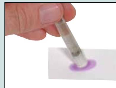
Applying reagent to non-destructive contact transfer.
