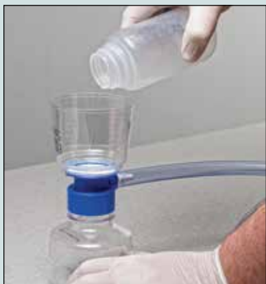
After area of interest is swept for DNA, pour the collected buffer solution through the filter, seal filter in provided breathable pouch with integrity tape, and send to lab for analysis.
