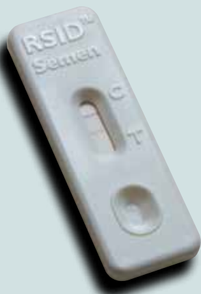
Results of the Semen, Saliva & Blood Detection Field Tests are fleeting and should be photographed immediately for documentation purposes.
