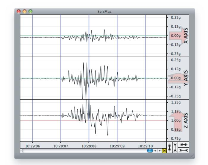
**SeisMac** - The ShakeMapple leverages the Sudden Motion Sensor Library and sensor calibration tool provided by the author of the SeisMac application. The SeisMac application provides a continuous display of the Apple laptop embedded sensor data.
