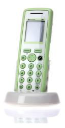
For correct charging, be sure the room temperature is between 0°C and 40°C. Do not place the handset in direct sunlight. The battery has a built-in heat sensor which will stop charging if the battery temperature is too high.
