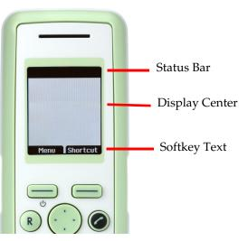
The display is divided in three parts: **Status bar**, **Display center** and **Softkey Text** (see figure above).
