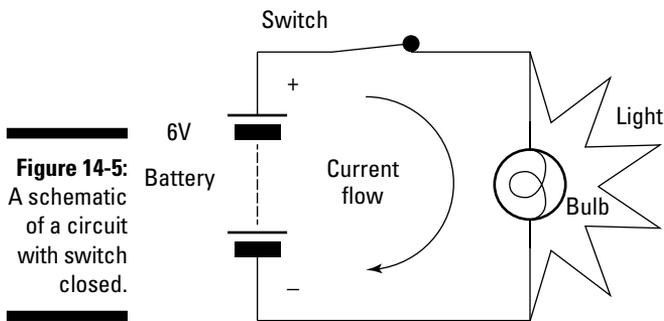
**Figure 14-5:** A schematic of a circuit with switch closed.
