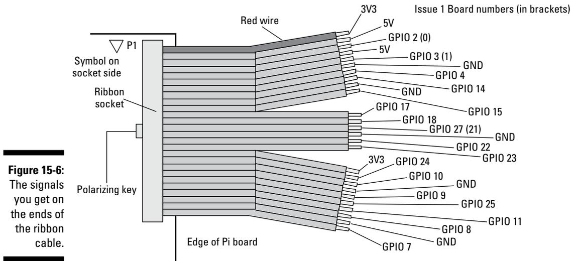
**Figure 15-6:** The signals you get on the ends of the ribbon cable.
