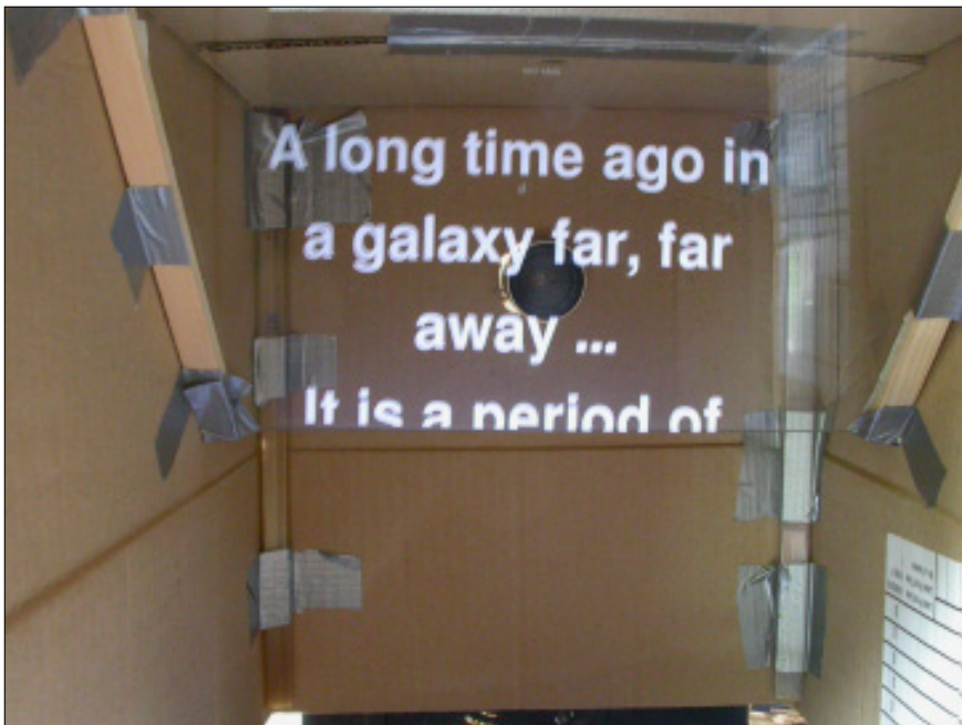
FIGURE 4-8: A closeup of the autocue, showing double reflections.
