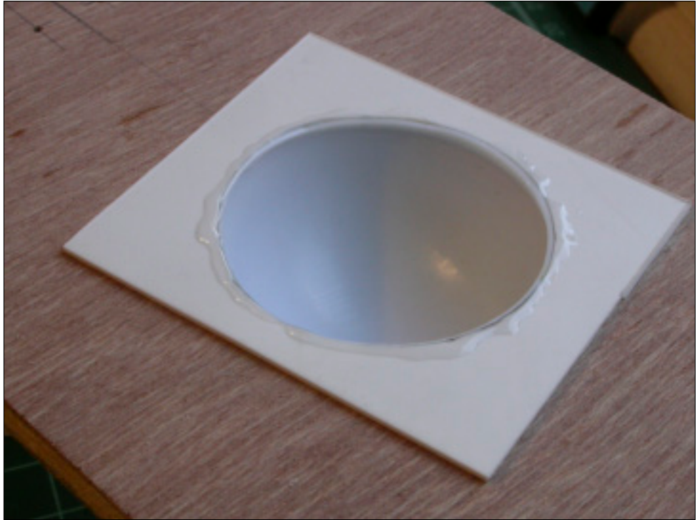
FIGURE 8-11: The ball and supporting base resting on the underside of the box's lid.
