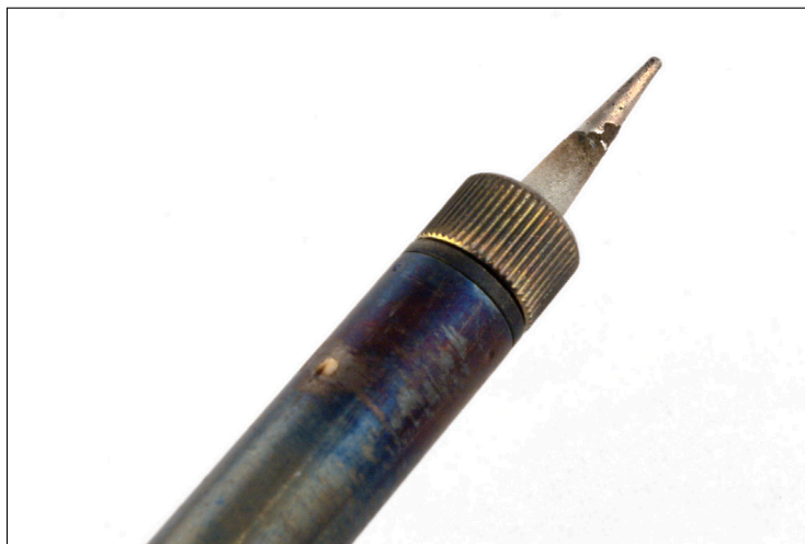
FIGURE 13-5: A soldering iron tip that is in the process of being tinned with solder
