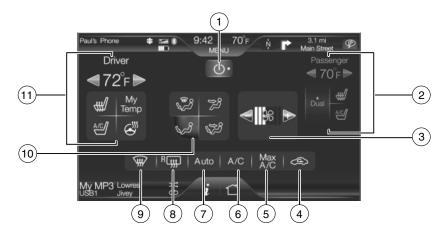
1. **() (Power):** Touch to activate/deactivate the system. Outside air cannot enter the vehicle when the system is off.
