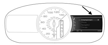
Your vehicle may have an infotainment display located on the right side of your instrument cluster. The display allows you to view and make minor adjustments to your active modes without taking your hands off the wheel. For example:
