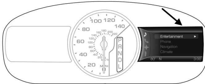
Your vehicle may have an infotainment display located on the right side of your instrument cluster. The display allows you to view and make minor adjustments to your active modes without taking your hands off the wheel. For example:
