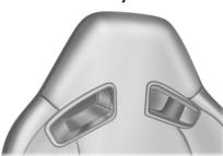
The non-adjustable head restraints consist of a trimmed foam covering over the upper structure of the seatback.
