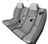
To lower the seatback(s) from inside the vehicle, be sure the head restraint is in the upright position, pull the strap to release the seatback and then fold the seatback down.
