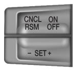
The speed controls are located on the steering wheel.
