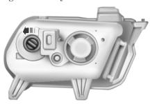
4. Rotate the socket counterclockwise and remove from the lamp assembly.
