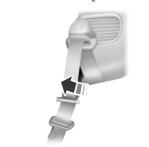
Rotate the presenter arm toward the front of the vehicle until it locks into place. This allows easier access to the front safety belt for the front seat occupant.
