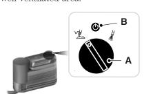
7. Turn dial (A) counterclockwise to the sealant position. Turn on the kit by pressing the on button (B).
