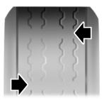
When the tread is worn down to 1/16th of an inch (2 mm), tires must be replaced to help prevent your vehicle from skidding and hydroplaning. Built-in treadwear indicators, or "wear bars", which look like narrow strips of smooth rubber across the tread will appear on the tire when the tread is worn down to 1/16th of an inch (2 mm).
