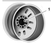
**Note:** Inspect the wheel pilot hole (1) and mounting surface prior to installation. Remove any visible corrosion or loose particles.
