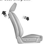
Use the seatback release to fold the back of the front seat forward for rear seat access. This release handle is located on the upper back of the front seat. The seatback locks automatically when returned to the normal position.
