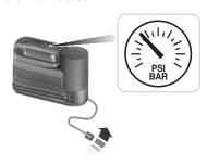
4. Adjust the tire to the recommended inflation pressure from the tire label located on the driver's door or door jamb area.
