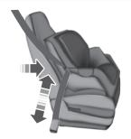
10. Before placing the child in the seat, forcibly move the seat forward and back to make sure the seat is securely held in place.
