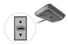
4. Press and hold the convertible top switch on the overhead console until the windows are completely down and the top is completely stored.
