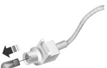
5. Carefully pull the bulb straight out of socket.
