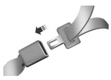
4. Insert the belt tongue into the proper buckle (the buckle closest to the direction the tongue is coming from) for that seating position until you hear a snap and feel the latch engage. Make sure the tongue is latched securely by pulling on it.
