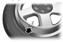
**Note:** Each road tire is equipped with a tire pressure sensor located inside the tire and wheel assembly cavity. The pressure sensor is attached to the valve stem. The pressure sensor is covered by the tire and is not visible unless the tire is removed. Care must be taken when changing the tire to avoid damaging the sensor.
