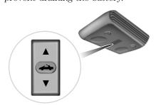
2. Press and hold the convertible top switch until the windows lower completely and the top unfolds and moves forward toward the windshield header.
