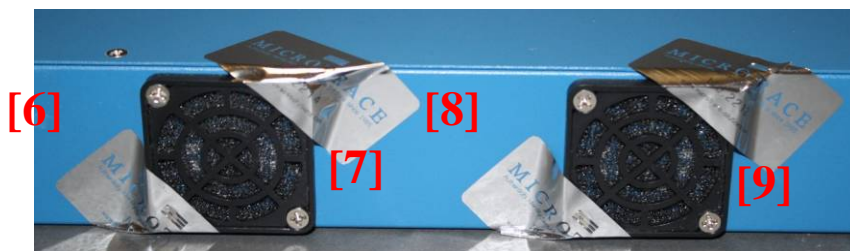
Figure 16 - PA-500 Rear Tamper Seal Placement (4)
