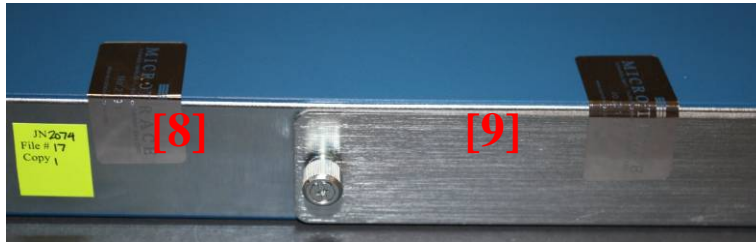
Figure 20 - PA-2000 Series Rear Tamper Seal Placement (2)
