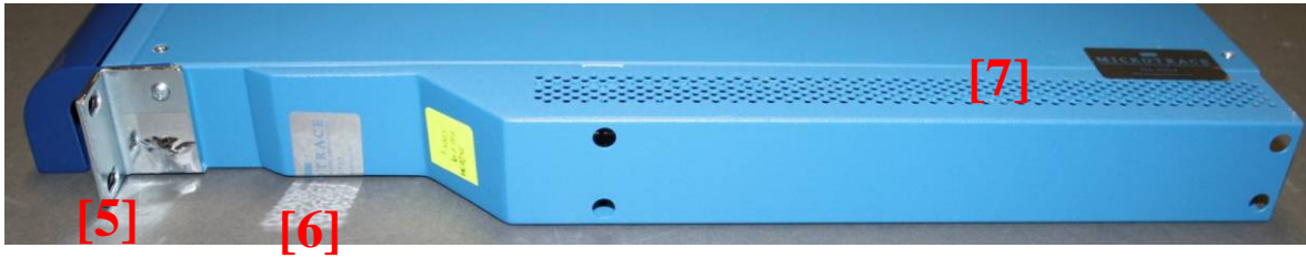
Figure 19 - PA-2000 Series Right Side Tamper Seal Placement (3)
