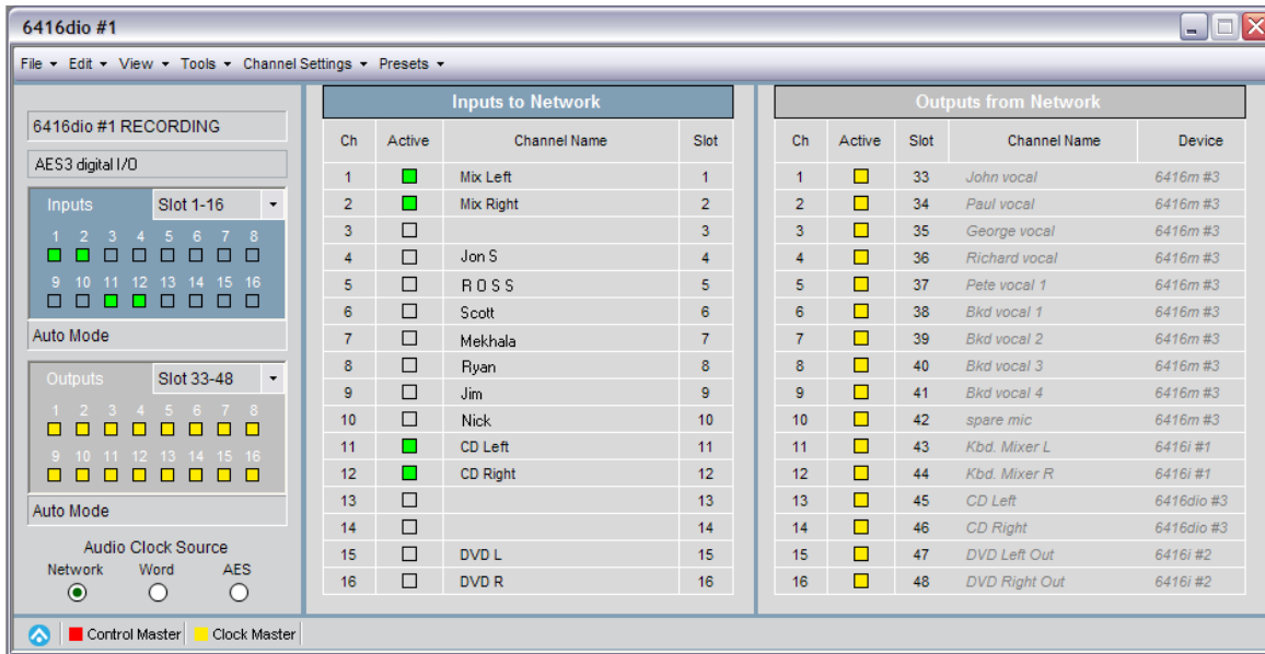
The Inputs and Outputs view for the 6416Y2 card
