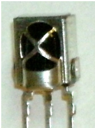
Figure 26-1. The VS1838B PIN photodiode
