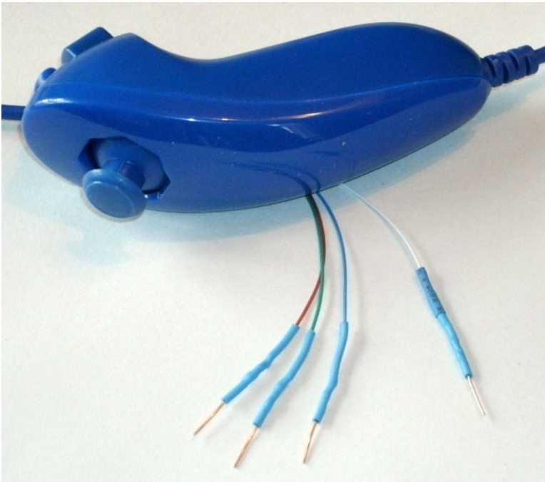
Figure 24-1. Nunchuk with wire ends
