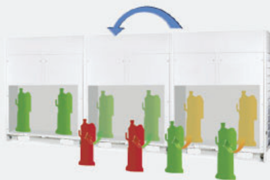
Start backup operation
