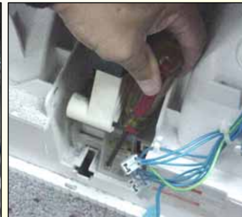
Unscrew pump cover screw
