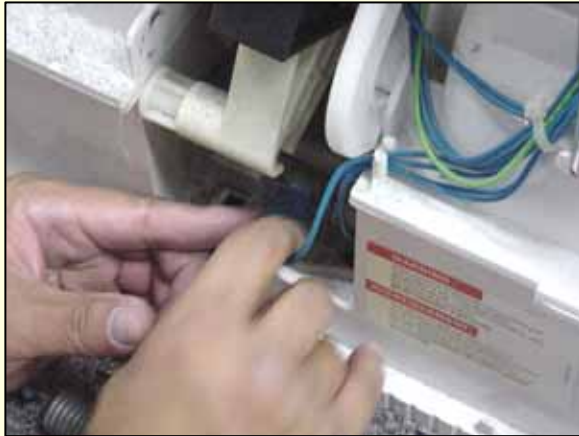
Disconnect drain pump wires
