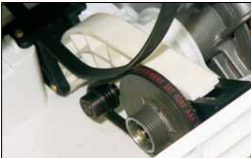
Replacing drive belt
