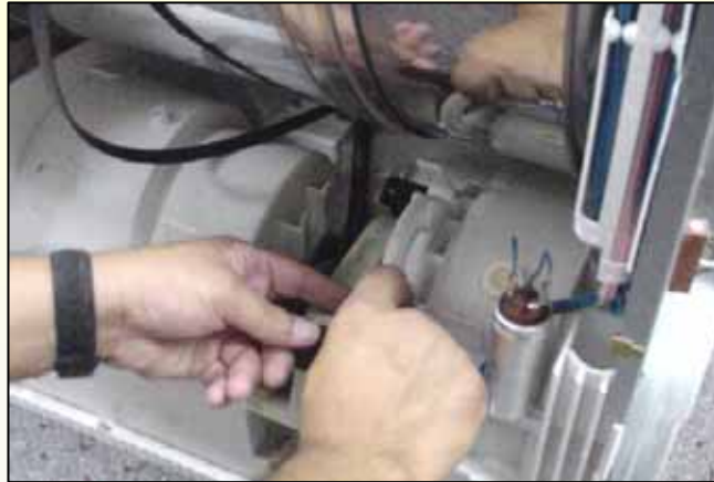
Slide drive belt off pulley
