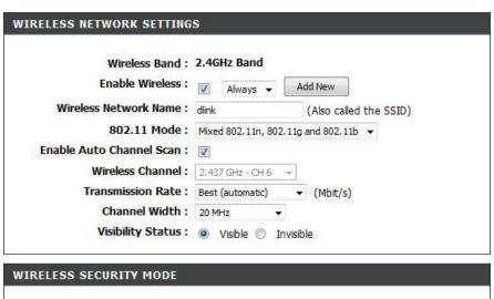
To protect your privacy you can configure wireless security features. This device supports three wireless security modes, including WEP, WPA-Personal, and WPA-Enterprise. WEP is the original wireless encryption standard. WPA provides a higher level of security. WPA-Personal does not require an authentication server. The WPA-Enterprise option requires an external RADIUS server.
