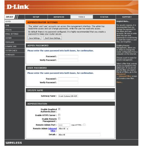
**Remote Admin** Example: http://x.x.x.x:8080 whereas x.x.x.x is the Internet IP address of the DIR-825 and 8080 is the port used for the **Inbound Filter:** Web Management interface. If you have enabled **HTTPS Server** and checked **Use HTTPS**, you must enter **https://** as part of the URL to access the router remotely.
