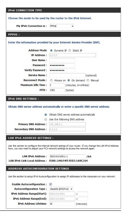
**Enable Autoconfiguration:** Check to enable the Autoconfiguration feature.
