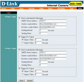
These fields control Input Trigger 1 and Trigger 2. Each Input trigger can trigger either or both Output triggers.
