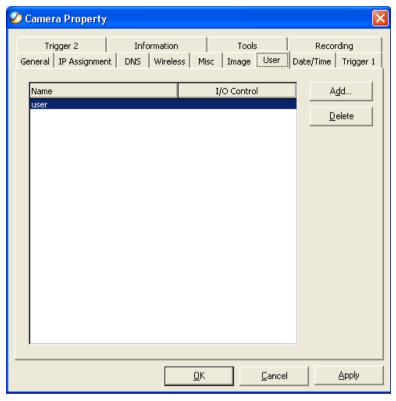
To add a user click on the **Add** icon and the **Add User** dialog box will appear. Enter the **User Name** and **Password** into the specific field. Select the I/O Output Control to give users the privilege of accessing the I/O Output Control.
