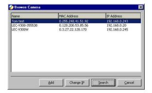
Highlight the camera you wish to add and click on **Add**. The **Add Camera** dialog box will appear once again with the IP Address entered. Click on **Add**. The camera will be automatically added into the IPView list view format.
