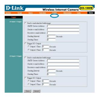
The default setting for the I/O Trigger functions is "disabled." You must enable the I/O Trigger first before the Triggers will perform.
