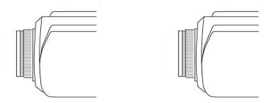
The Internet Camera features an exchangeable C/CS-type lens that can be used for different applications as necessary. It supports rotational focus control so the lens can be adjusted to focus under normal and stable conditions to maximize the image quality of the Internet Camera.
