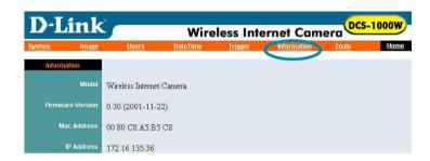
The Information table provides detailed information about the Internet Camera such as the Model Name, Firmware Version, Mac Address, and IP Address.
