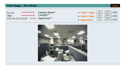
**Camera Name\*** - The Camera name will be display when the Camera Name field is entered in the Web Configuration setting under "**System**"
