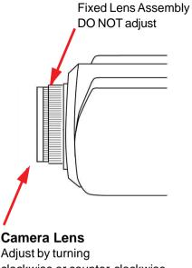
Adjust by turning clockwise or counter-clockwise
