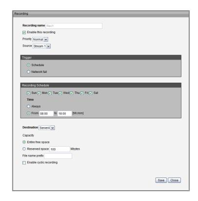
**Enable cyclic recording:** If you check this box, when the maximum capacity is reached, the oldest file will be overwritten by the latest one. The reserved amount is reserved for cyclic recording to prevent malfunction. This value must be larger than 15 Mbytes.
