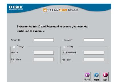
Select **DHCP** if your camera obtains an IP address automatically when it boots up. Select **Static IP** if the camera will use the same IP address each time it is started.
