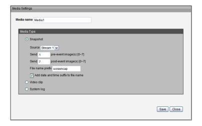
**Video clip:** Select to send video clips when a trigger is activated.
