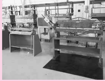
Jet Mdl BP-1648 48" Sheet Metal Finger Brake, 16 Gauge Capacity Berkroy Mdl B-936 36" Sheet Metal Finger Brake
