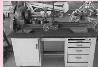
Craftsman Mdl 101-077403 Bench Top Lathe, 13" Swing, 3-1/4 Hollow Spindle, 3 & 4 Jaw Chucks, 36" Between Centers w/Various Tooling 12" Metal Cutoff Saw
