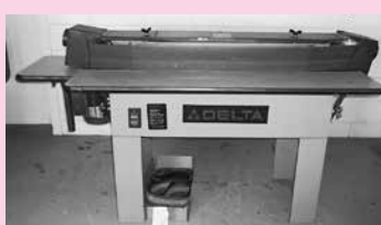
Delta Mdl 31-390 6" Edge Sander, 38" Sanding Area, 6" x 132" Belt, 2-HP, 1-Phase Motor 8" Disc Sander, 1-HP Motor Dayton Mdl 12773A 4" Belt Sander Delta Rockwell Mdl 101-6402 6" Belt Sander, 3/4 HP Motor Jet Mdl JDS-20-1 20" Disc Sander, 2-HP, 1-Phase Motor
