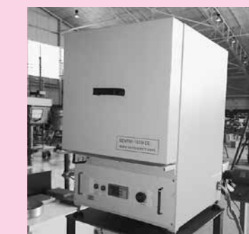
Sentro Tech ST-1200-7812-AG High Temp Heat Treat Furnace, 1,200° C Max Temp, Chamber Size 7" x 8" x 12", Digital Temp Controller
