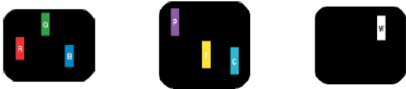
One lit red, green or blue sub pixel Two adjacent lit sub pixels: - Red + Blue = Purple - Red + Green = Yellow - Green + Blue = Cyan (Light Blue) Three adjacent lit sub pixels (one white pixel)
