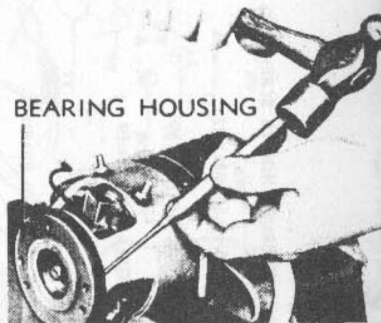
D—REMOVE BEARING HOUSING WITH DRIFT OR PULLER.
