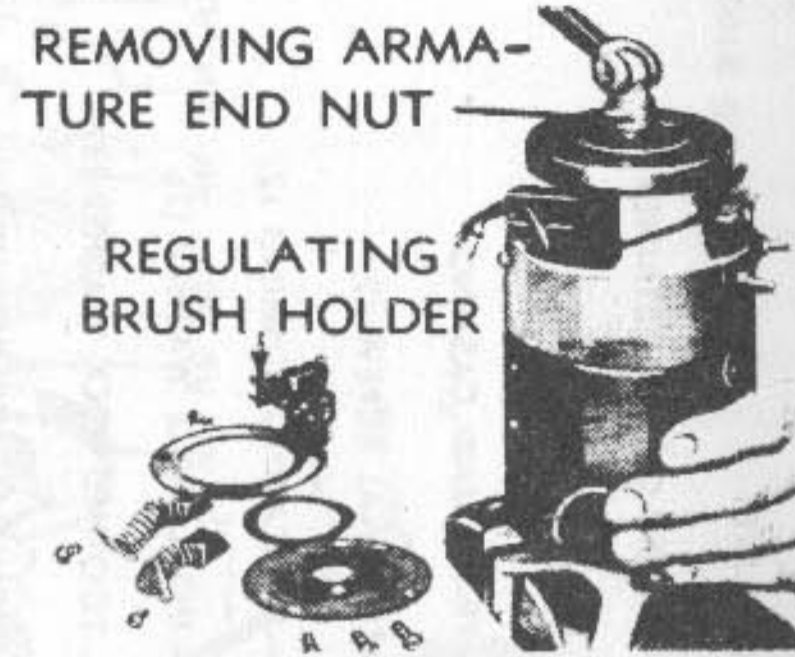
B—REMOVE ARMATURE END NUT. BRUSHES REMOVED.
