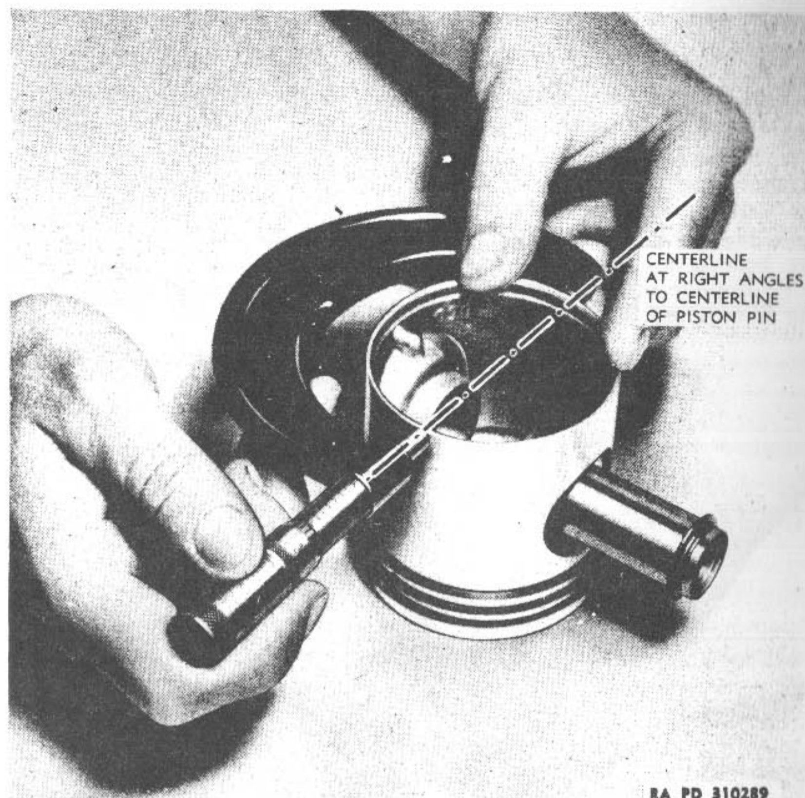
Figure 15—Measuring Piston with Micrometer Calipers (41-C-307)
