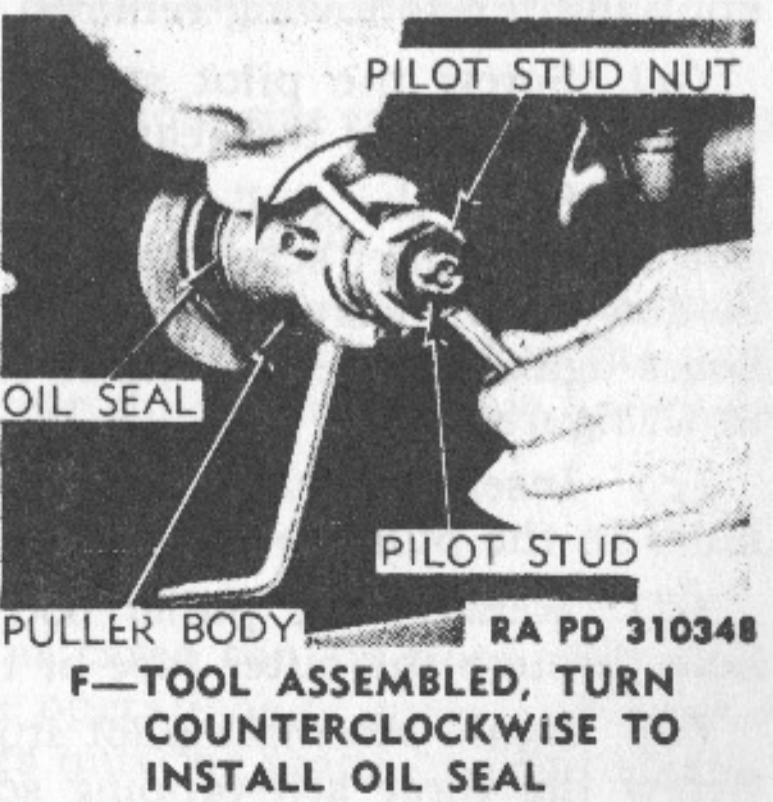
Figure 101—Removing Clutch Gear Oil Seal with Tool (41-R-2389-47)
