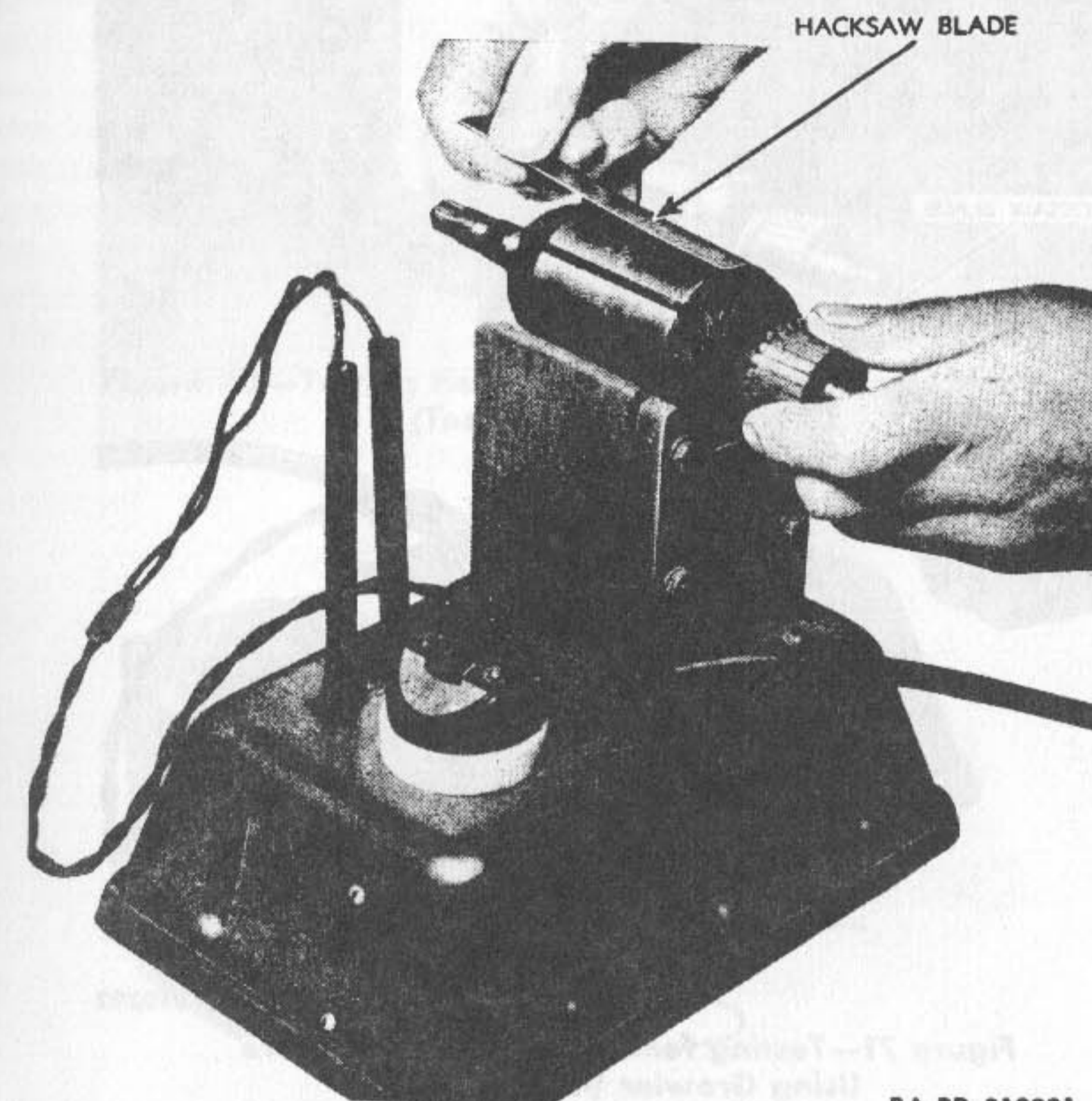
Figure 70—Testing for Shorted Armature Coils Using Growler (41-G-5940)
