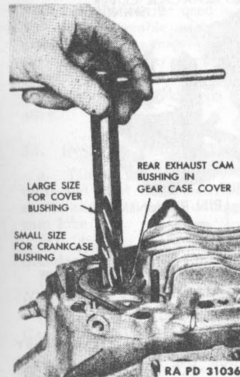
Figure 48—Line-reaming Oil Pump Drive Shaft Bushing and Crankcase Rear Exhaust Cam Bushing with Reamer (41-R-2303)
