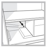
special discharge outlet (see diagram) where the heat produced by the compressor causes it to evaporate. It is necessary to clean
