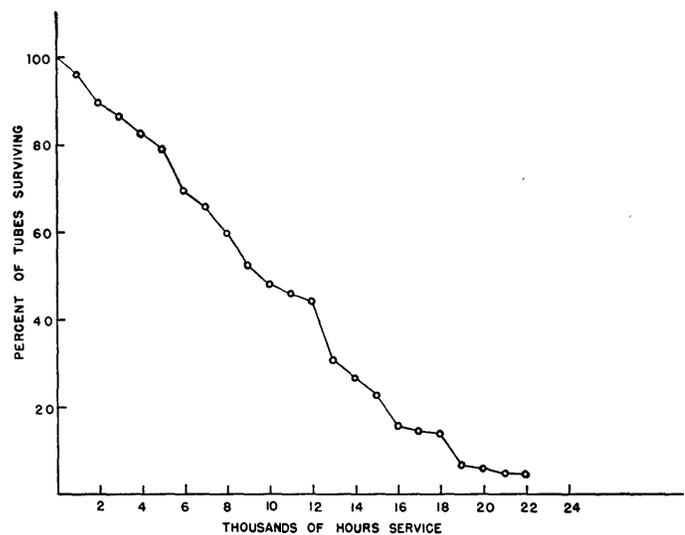
Fig. 2—Over-all tube survival versus time in service for 1,775 type 6AN5 tubes.
