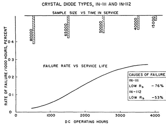
Fig. 9—Failure rate vs service life for crystal diode types 1N111 and 1N112.
