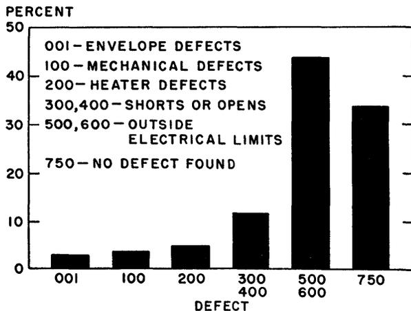
Fig. 10—Defect distribution of tubes removed from shipborne equipments.
