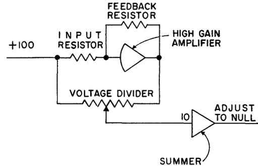
Fig. 2—Amplifier gain calibration circuit.
