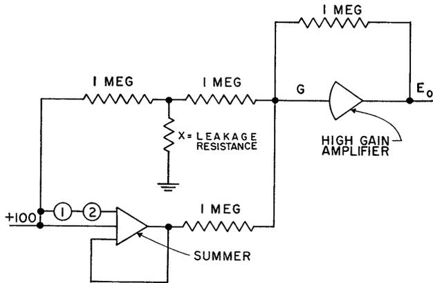
Fig. 4—Circuit for measuring interconsole leakage resistance.
