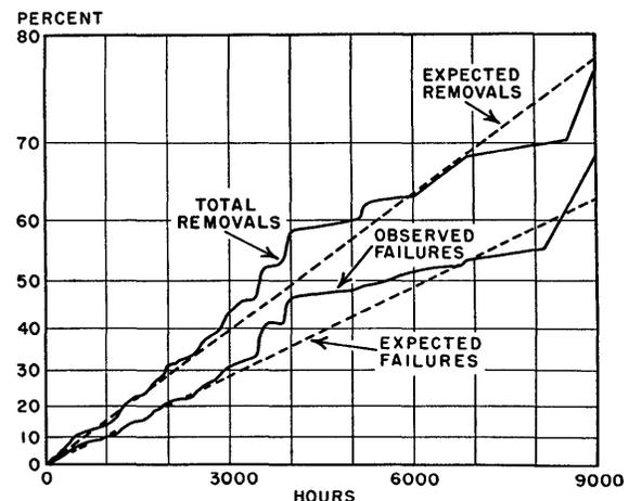
Fig. 11—Tube mortality with time, shipborne equipments.
