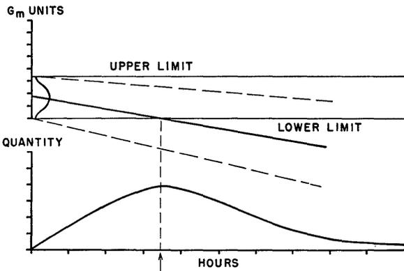
Fig. 4—Theoretical plot of expected tube removals based on  $G_m$  deterioration with time.
