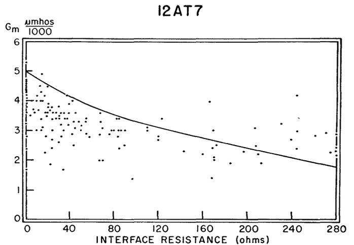
Fig. 9—12AT7 removals from land-based teletype equipment: cathode interface resistance vs  $G_m$ .
