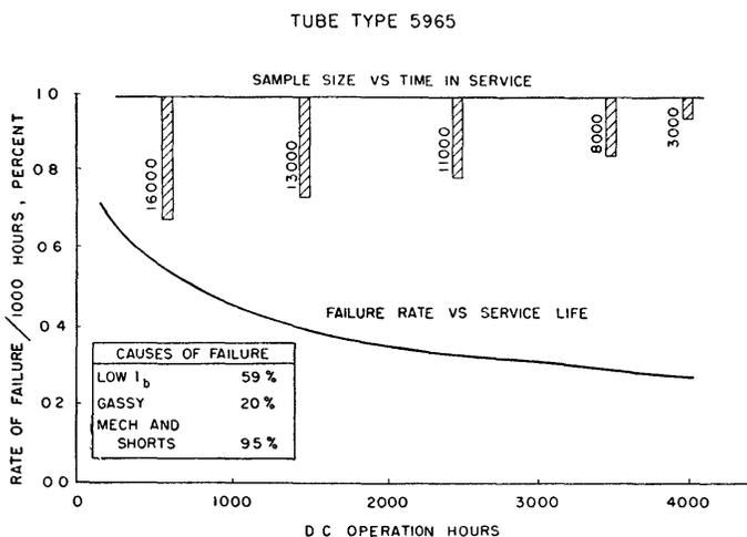
Fig. 8—Failure rate vs service life for tube type 5965.
