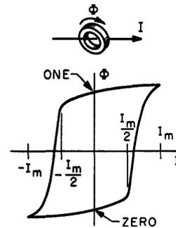
Fig. 1—Flux-current characteristic of ferrite toroid.
