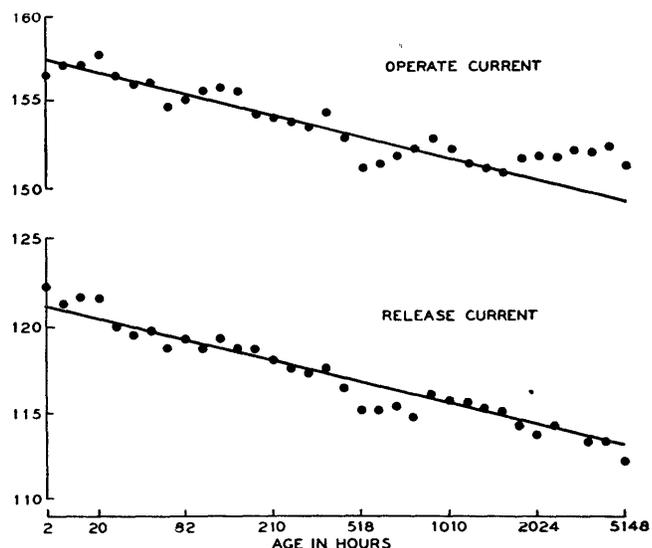
Fig. 4—Operate and release currents—average of ten relays.
