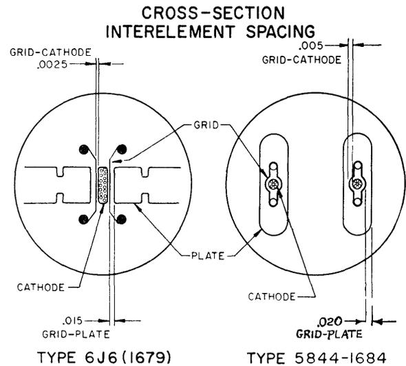
Fig. 6—Comparison of interelement spacing in 6J6 and 5844.
