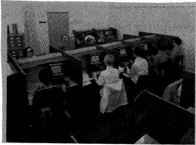
Figure 1—The PLATO III system provides each student with an electronic keyset as a means of communicating with the computer and a television display for viewing information selected or generated by the computer
