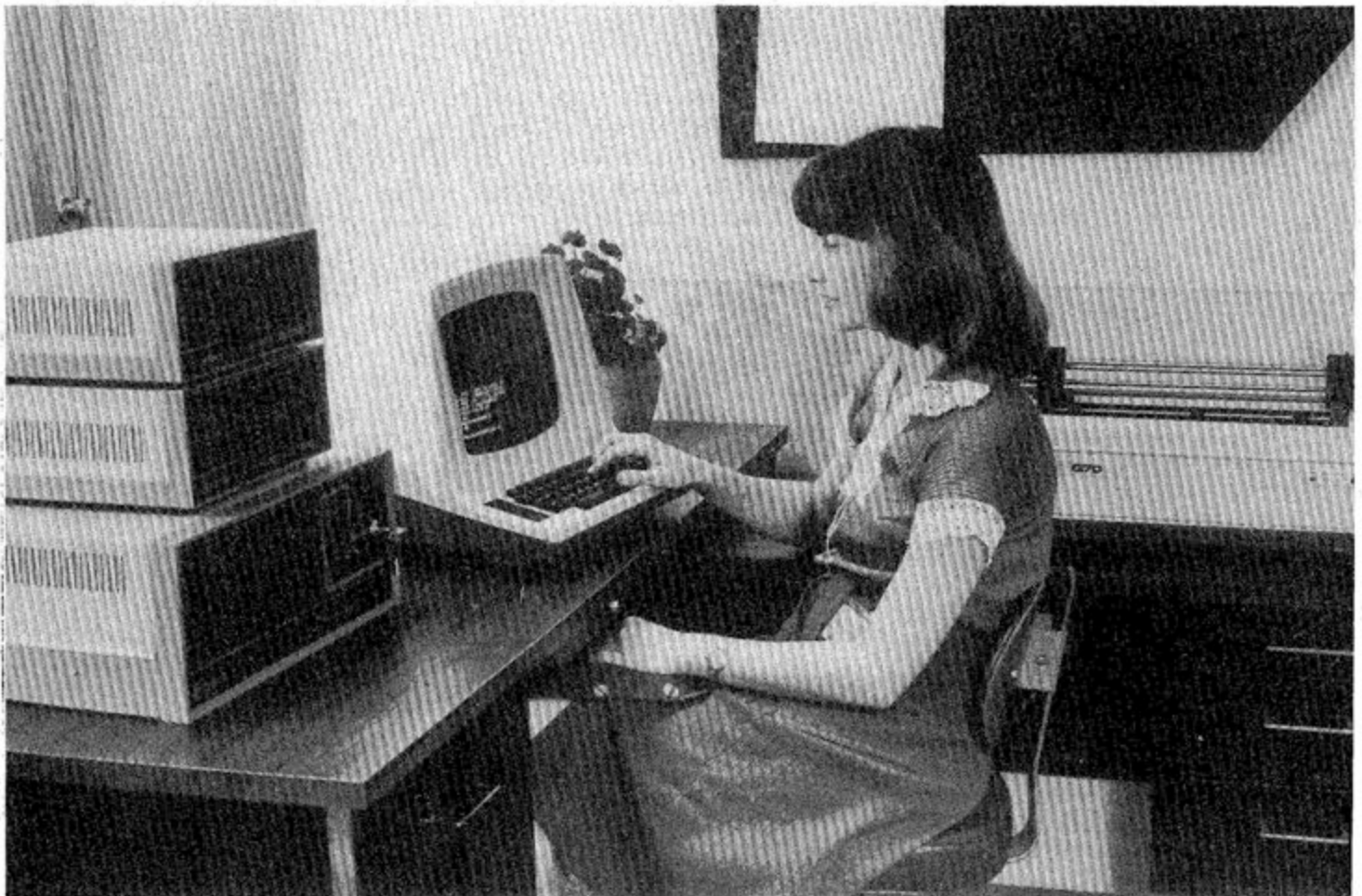
Altair system featuring 8800b Turnkey Model, dual Altair Minidisks, LSI ADM-3 CRT and Q70 Line Printer.
